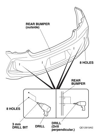
Using a 24 mm hole saw, enlarge the outboard (left and right corner sensor) bumper holes by drilling the lower 3 mm holes. Remove any burrs.
