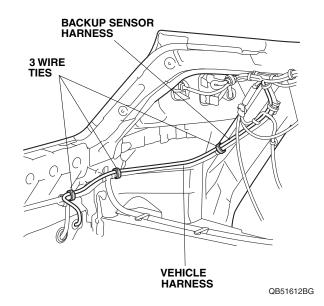
39. If equipped with vehicle another harness, install the wire tie with holder to the backup sensor harness8-pin connector, and secure it to the vehicle harness.Go to step 41.
