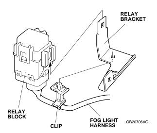
24. Secure the clip from the fog light harness to the relay bracket.
