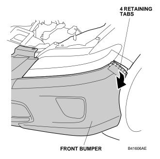
Release the four retaining tabs on each side.
