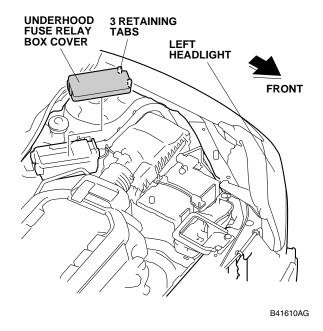
38. Plug the 15A fuse into the underhood fuse relay box.
