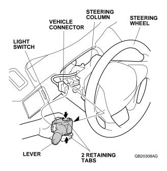
Push in on the two retaining tabs, slide the light switch out, and remove it from the steering column. Do not pull on the lever. Install the new light switch to the steering column.
