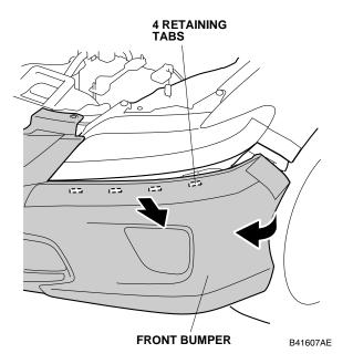
• Remove the two clips. With the help of an assistant, remove the front bumper.
