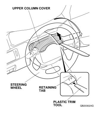
3. Turn the steering wheel 180° counterclockwise. Using a plastic trim tool, release the retaining tab.
