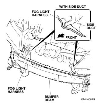
32. Align the green tape on the fog light harness with the vehicle clip, and secure the fog light harness to the vehicle harness with one wire tie.
