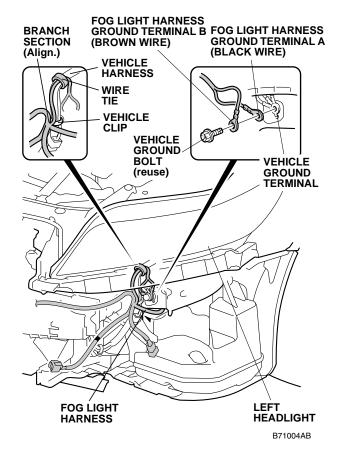
27. Secure the fog light harness to the vehicle harness with one wire tie at the location shown.
