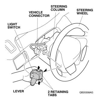
9. Push in on the two retaining tabs, slide the light switch out, and remove it from the steering column. Do not pull on the lever.
