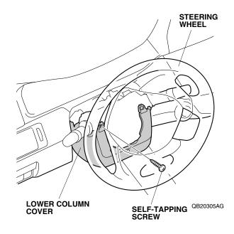
6. Turn the steering wheel 180° clockwise, and remove the other one self-tapping screw from the lower column cover.
