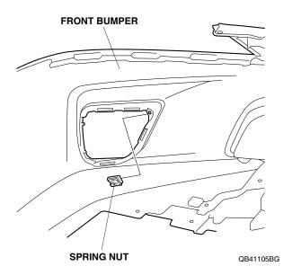
19. Install the left fog light to the front bumper with two hooks, four retaining tabs and one 5 x 20 mm self-tapping screw.
