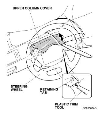
3. Turn the steering wheel 180° counterclockwise. Using a plastic trim tool, release the retaining tab.
