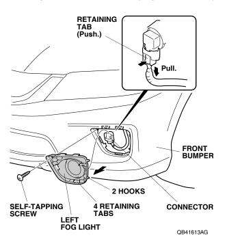
2. Remove the bulb from the fog light as shown.
