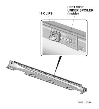
17. Attach masking tape to protect the left side under spoiler.
