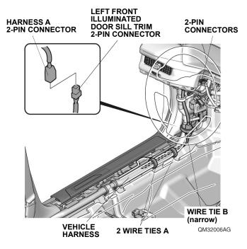
57. Secure the left front illuminated door sill trim harness and connectors.
