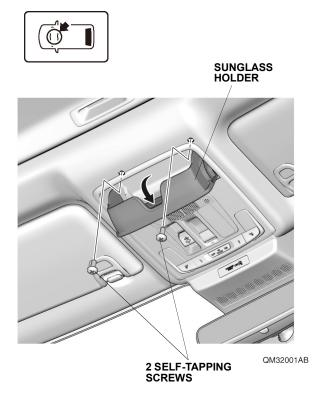
4. Remove the roof module.
