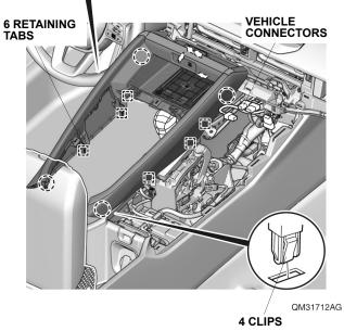
18. Remove the passenger's dashboard under cover.
