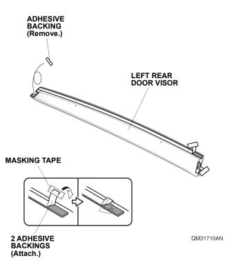
15. Remove the adhesive backing.
