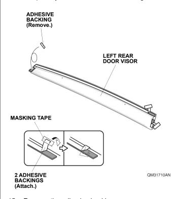
15. Remove the adhesive backing.
