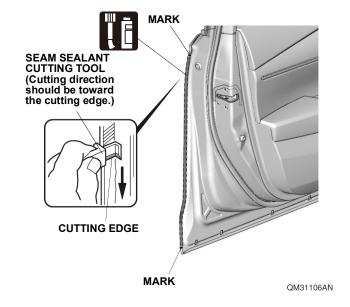
9. Temporarily install the left rear door edge guard.
