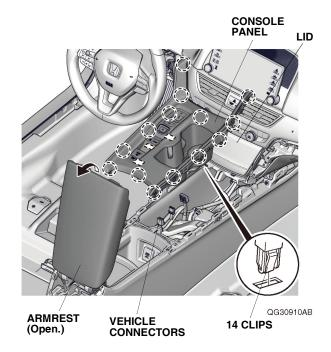
29. Remove the dashboard center trim and unplug the vehicle connectors.
