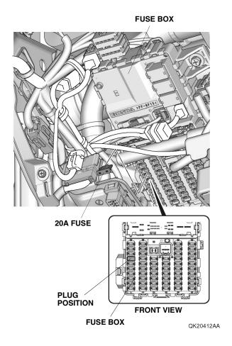
78. Using isopropyl alcohol on a shop towel, thoroughly clean the fuse label where the fuse label B will attach. Attach the fuse label B (20A OPTION FUSE) to the fuse label on the driver's kick panel as shown.
