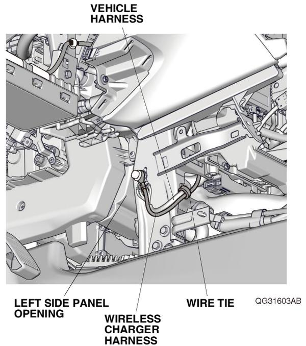
63. Remove the vehicle ground bolt, and secure the wireless charger harness ground terminal to the vehicle ground terminals with vehicle ground bolt. NOTE: Do not put the ground terminal calkings on top of one another.
