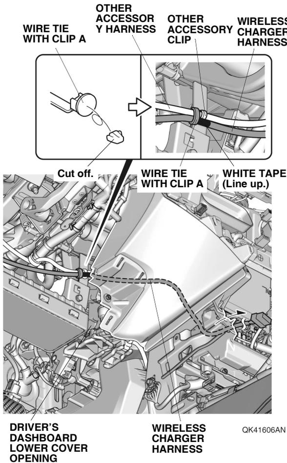
56. Line up the white tape on the wireless charger harness with the other accessory clip, and secure the wireless charger harness to the other accessory harness with one wire tie with clip A as shown.
