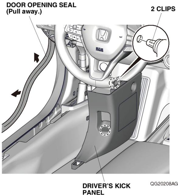
17. Remove the driver's inner dashboard trim and unplug the vehicle connector.
