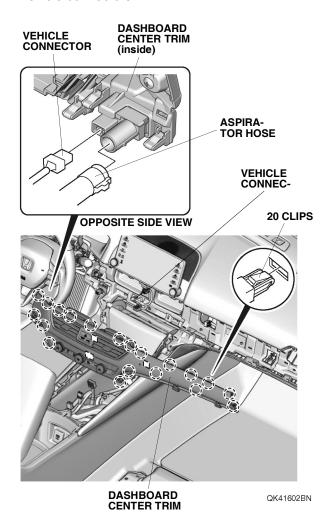
30. Remove the center pocket, and unplug the vehicle connectors.
