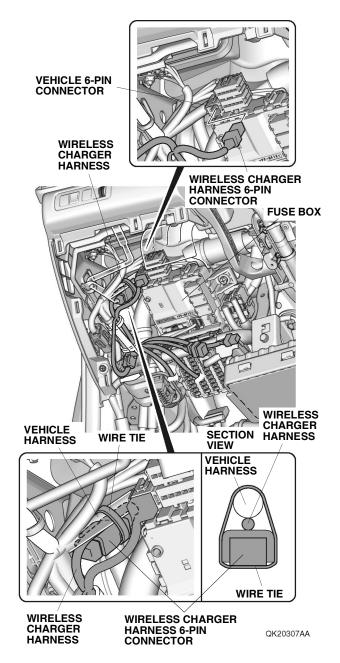
38. Secure the wireless charger harness 6-pin connector to the vehicle harness with one wire tie as shown. Go to step 47.
