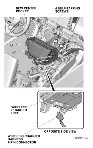
76. Install the new center pocket with four self-tapping screws removed in step 30.
