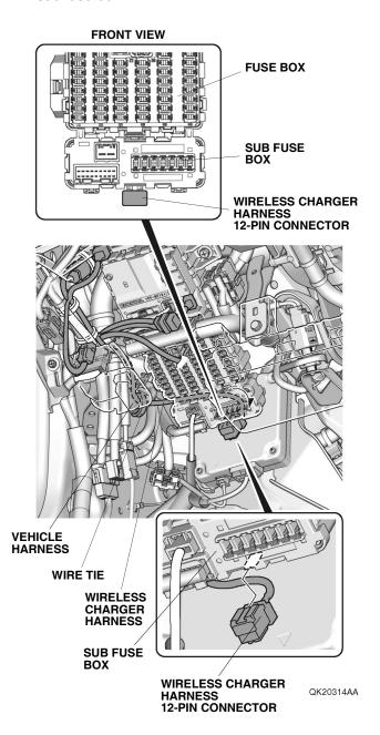
50. Secure the wireless charger harness to the vehicle harness with one wire tie. Go to step 53.
