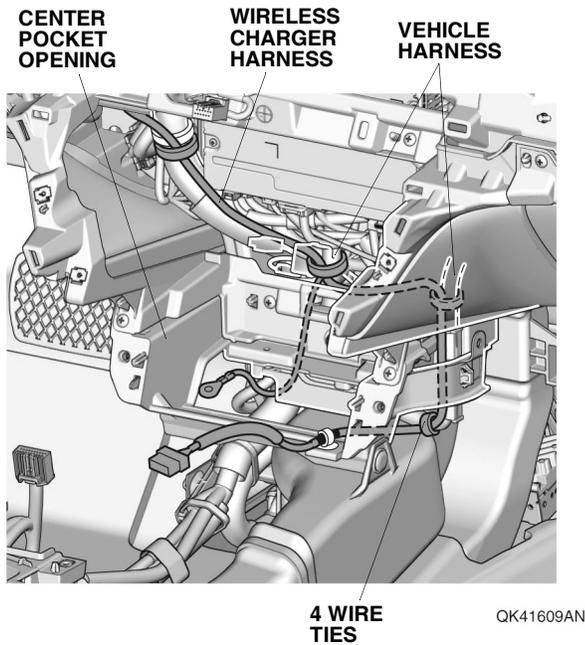
64. Secure the wireless charger harness to the vehicle harness with one wire tie.
