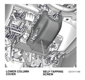
17. Remove the driver's inner dashboard trim and unplug the vehicle connector.
