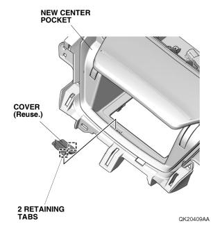
74. Install the wireless charger unit in the new center pocket with four retaining tabs and four self-tapping screws.
