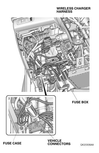
36. If the vehicle is equipped with another accessory harness, follow the plug-in order shown below.
