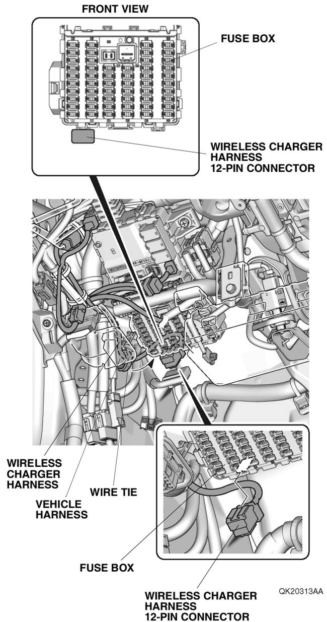
52. Secure the wireless charger harness to the vehicle harness with one wire tie.
