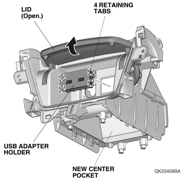
71. Install the housing in the new center pocket with eight retaining tabs.
