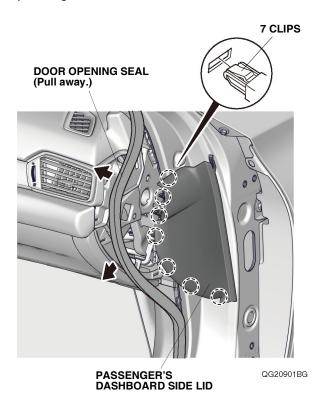
Open the glove box and remove the passenger's trim panel. Close the glove box.
