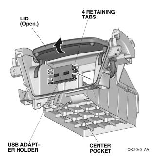
66. Open the housing cover, and remove the accessory power socket.
