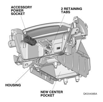
73. Install the cover removed in step 21 in the new center pocket with two retaining tabs.
