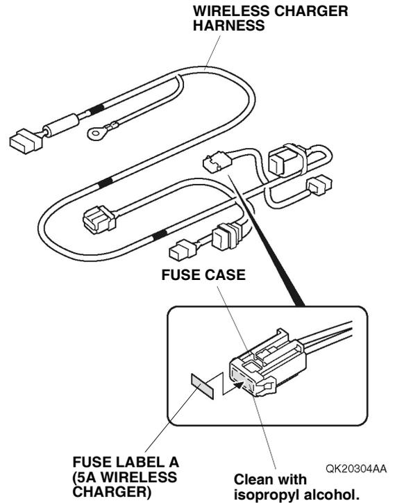
34. Line up the branch section of the wireless charger harness with the vehicle clip. Secure the wireless charger harness to the vehicle harness with two wire ties.
