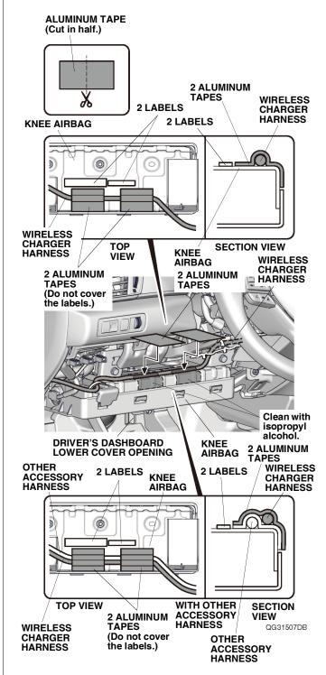
58. Using scissors, cut one piece of aluminum tape in half and secure the wireless charger harness to the knee airbag with two pieces of aluminum tape as shown. If the vehicle is already equipped with another accessory harness, secure the wireless charger harness to the knee airbag with two pieces of aluminum tape as shown.
