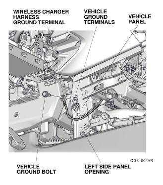
64. Secure the wireless charger harness to the vehicle harness with one wire tie.
