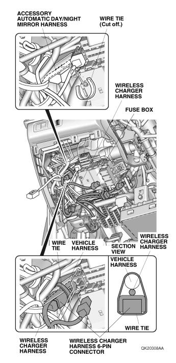
40. Secure the wireless charger harness 6-pin connector to the vehicle harness with one wire tie as shown.
