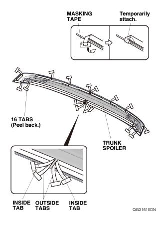
Place the trunk spoiler on the trunk lid. Insert the two bolts into the holes in the trunk lid first, then insert the two pins. Do not apply excessive pressure.
