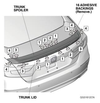
21. Using your hand, firmly press the trunk spoiler against the trunk lid.
