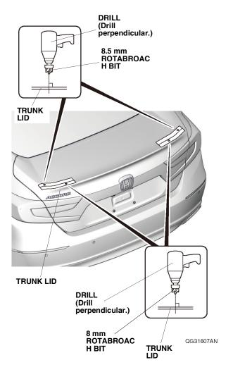
10. While wearing eye protection, use an 8 mm Rotabroach bit to drill the two inner 3 mm holes as shown.
