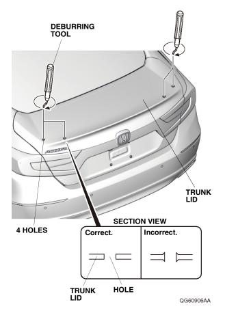
13. Apply touch-up paint to the edges of the holes, and allow the touch-up paint to dry.
