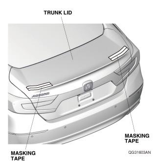
Place the template on the left side of the trunk lid, and line up the template with the trunk lid as shown. Tape the template to the trunk lid with masking tape.
