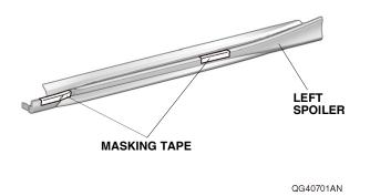
9. Install the left spoiler to the vehicle panel with the 13 clips. Remove the masking tape.
