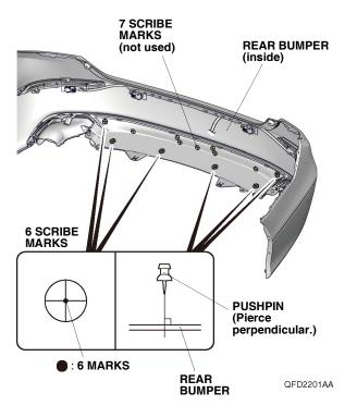
While wearing eye protection, drill the six pierced marks to 8 mm. First, drill with a 3 mm drill bit, then follow with a 6 mm drill bit, and finish with an 8 mm drill bit.
