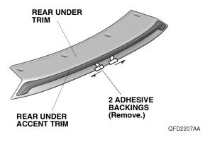
10. Using a rubber roller, apply firm pressure against the rear under accent trim and roll from one end to the other.
