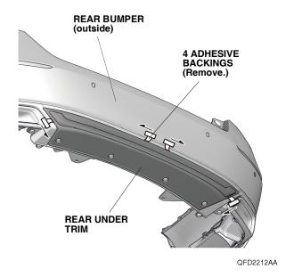
15. Using a rubber roller, apply firm pressure against the rear under trim and roll from one end to the other. NOTE: Apply firm pressure, especially at the ends.
