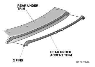
9. While applying light pressure against the rear under accent trim, carefully remove the taped adhesive backings.
