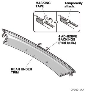
13. Line up the rear under trim with the rear bumper as shown. Loosely install the rear under trim to the rear bumper with four clips, two washers, and two selftapping screws.
