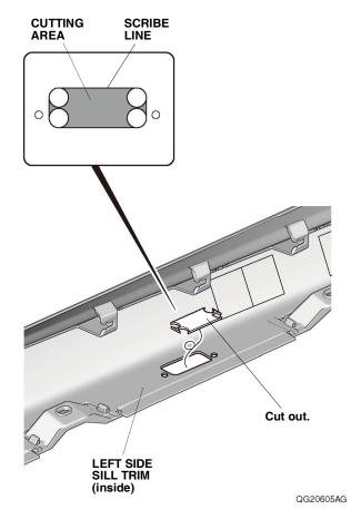
63. Install the light and light trim to the left side sill trim with two self-tapping screws.
