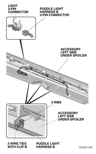
72. Secure the puddle light harness B to the ribs on the accessory left side under spoiler with three wire ties with clip B.
