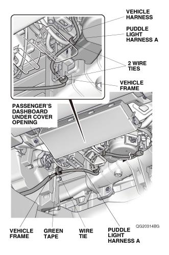
45. Secure puddle light harness A to the vehicle frame and vehicle harness with two wire ties.
