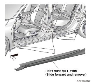
20. Remove the 13 clips from the vehicle panel.
