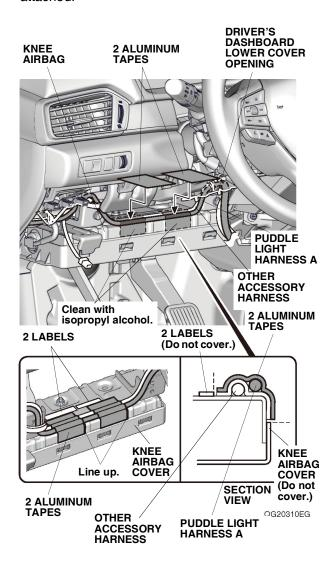
40. Secure puddle light harness A to the knee airbag with two pieces of aluminum tape as shown.
