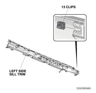
68. To prevent damage from hitting the doors while installing, apply masking tape to the left side sill trim.
