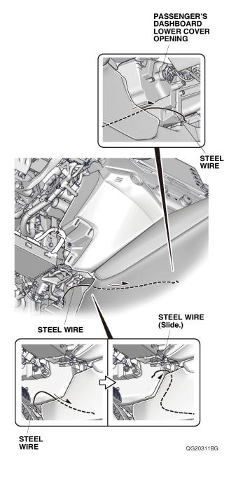
42. Attach the steel wire to puddle light harness A with masking tape as shown.
