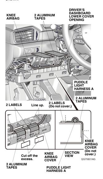
35. Using isopropyl alcohol on a shop towel, thoroughly clean the knee airbag where the aluminum tape will attached.
