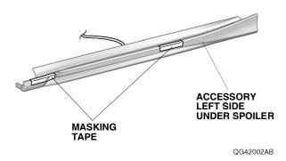
74. Install the accessory left side under spoiler to the vehicle. Remove the masking tape.
