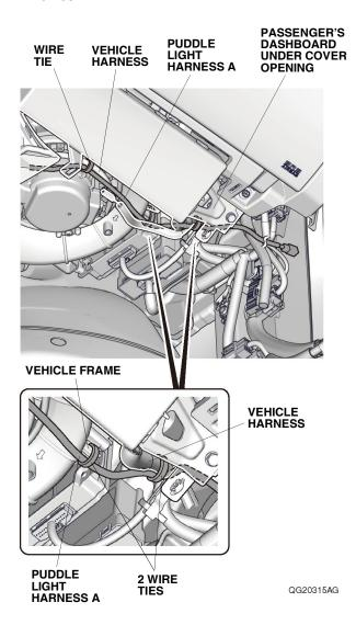
47. Route puddle light harness A along the vehicle harness, and secure it to the vehicle harness with one wire tie.
