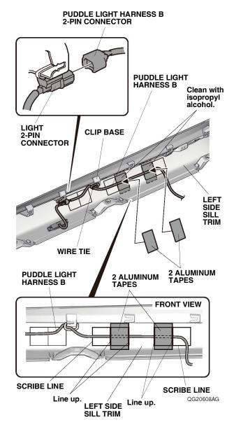
66. Using isopropyl alcohol on a shop towel, thoroughly clean the left side sill trim where the aluminum tape will attach. Secure puddle light harness B to the left side sill trim with two pieces of aluminum tape as shown.
