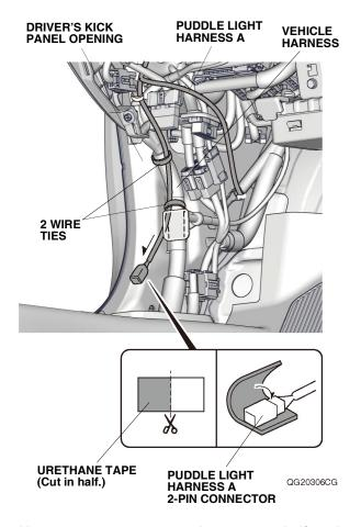
Using scissors, cut one urethane tape in half, and attach one piece around the puddle light harness A 2-pin connector.
