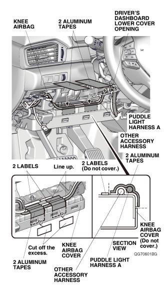
39. Using isopropyl alcohol on a shop towel, thoroughly clean the knee airbag where the aluminum tape will attached.
