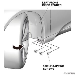
17. Remove the three self-tapping screws from the left front inner fender.
