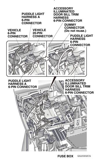
26. Remove the dummy connector from the puddle light harness A 6-pin connector. Plug the accessory illuminated door sill trim harness 6-pin connector into that connector. Go to step 29.
