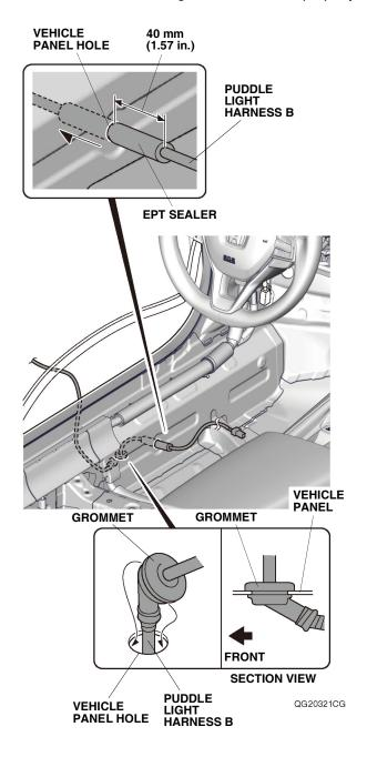
55. Route puddle light harness B along the vehicle harness. Plug the puddle light harness B 2-pin connector into the puddle light harness A 2-pin connector, and secure the 2-pin connectors to the vehicle harness with one wire tie as shown.
