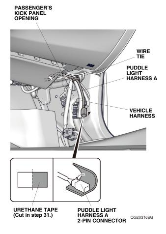
48. Attach one piece of urethane tape cut in step 31 around the puddle light harness A 2-pin connector.
