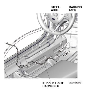
53. Push the grommet on puddle light harness B into the vehicle panel hole, and wrap it EPT sealer as shown.
