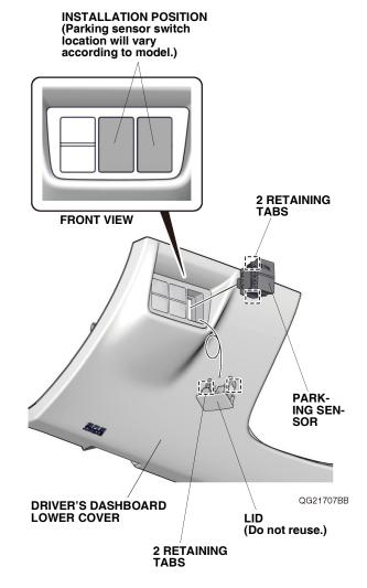
129. Install the parking sensor switch to the driver's dashboard lower cover.
