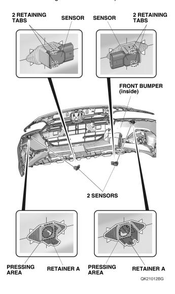
145. Remove the four adhesive backings, and firmly press the two retainers A against the front bumper. Install the two sensors.
