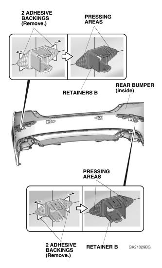
178. Remove the four adhesive backings, and firmly press the two retainers B against the rear bumper. Install the two sensors.
