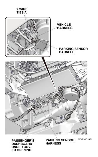
100. Route the parking sensor harness, and secure it to the vehicle harness and vehicle frame with two wire ties A.
