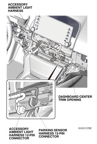
76. Secure the parking sensor harness to the vehicle harness and accessory ambient light harness with one wire tie A.
