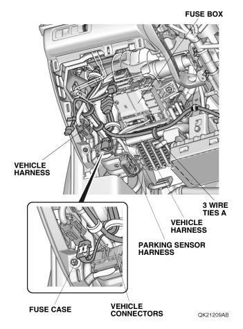
97. Secure the fuse case on the parking sensor harness to the vehicle connectors.
