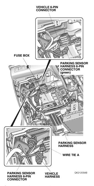
87. Secure the parking sensor harness 6-pin connector to the vehicle harness with one wire tie A. Go to step 96.
