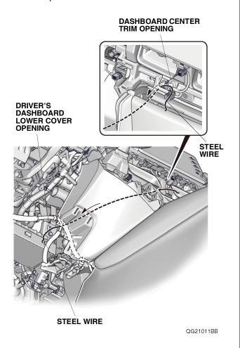
63. Attach the steel wire to the parking sensor harness with masking tape as shown.
