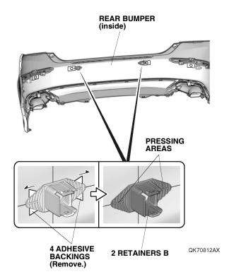
179. Make sure the four sensors are installed properly.
