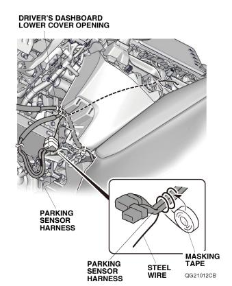
64. Route the parking sensor harness as shown. Remove the masking tape and steel wire.
