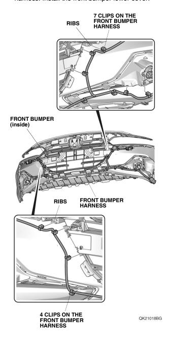
154. Using diagonal cutters, cut off the clip portion of one wire tie with clip A. Secure the front bumper harness to the vehicle harness with one wire tie with clip A. If the vehicle is not equipped with fog lights, attach one wire tie with clip A to the front bumper harness 4-pin connector as shown. Secure the front bumper harness 4-pin connector to the front bumper with one wire tie with clip A.
