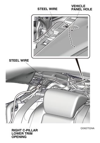
118. Attach the steel wire to the parking sensor harness with masking tape as shown.
