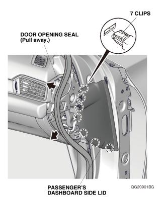
11. Remove the passenger's dashboard under cover.
