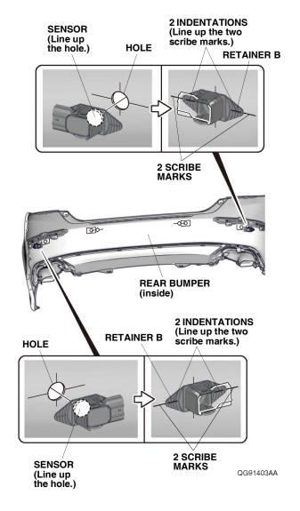
168. Line up the two sensors and two retainers B to the rear bumper as shown.
