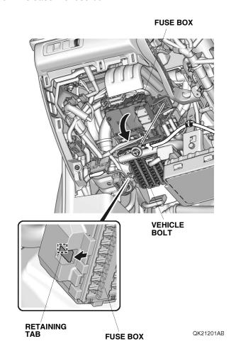
80. Route the parking sensor harness. Unplug the vehicle 20-pin connector, and plug the parking sensor harness 20-pin connector into the fuse box. Plug the vehicle 20-pin connector into the parking sensor harness 20-pin connector.
