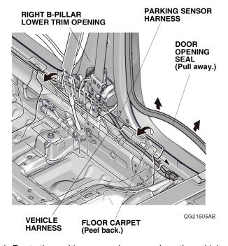
114. Route the parking sensor harness along the vehicle harness. 115. Secure the parking sensor harness to the vehicle harness with two wire ties A as shown.
