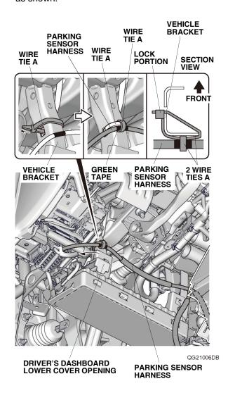
58. Attach one wire tie with clip B to the branch section of the parking sensor harness as shown. Secure the parking sensor harness to the vehicle bracket with one wire tie with clip B. Go to step 61.
