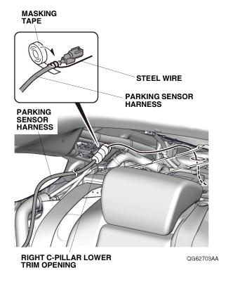
119. Route the parking sensor harness as shown. Remove the masking tape and steel wire.
