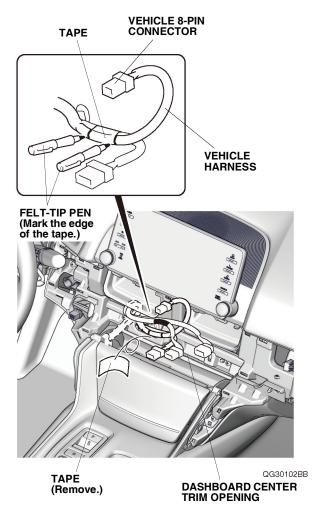
66. Remove the tape to free the vehicle harness.
