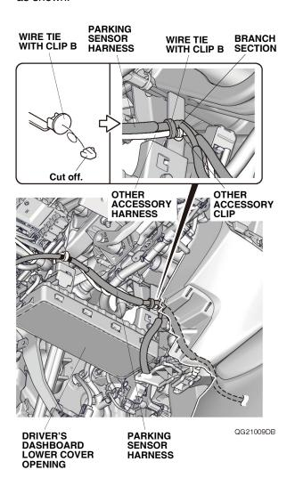
61. Secure the parking sensor harness to the vehicle frame with one wire tie with clip C as shown. If the vehicle is already equipped with another accessory harness, cut off the clip from that harness. Secure the parking sensor harness and other accessory harness to the vehicle frame with one wire tie with clip C.
