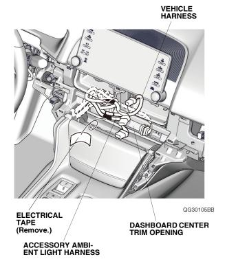
74. Line up the green tape on the parking sensor harness with the two marks on the vehicle harness, and secure the parking sensor harness and vehicle harness with electrical tape as shown.
