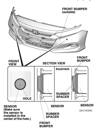
141. Using a felt-tip pen, mark the front bumper as shown.
