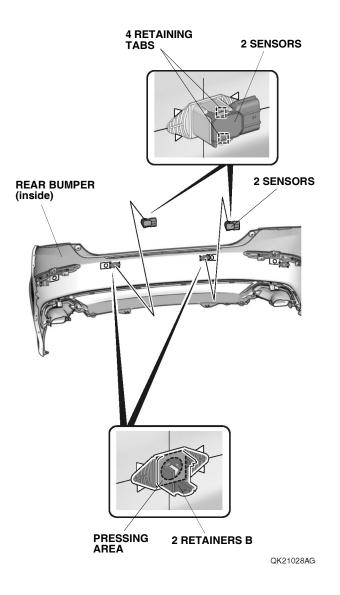
177. Remove the four adhesive backings, and firmly press the two retainers B against the rear bumper. Install the two sensors.
