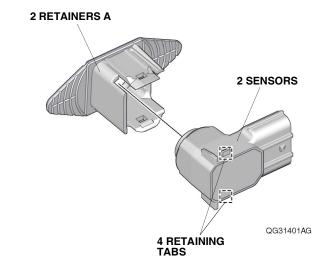
139. Line up the two sensors and two retainers A to the front bumper as shown.
