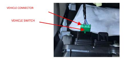
After connecting the parking sensor harness 5-pin connector into the parking sensor switch in step 130, make sure the vehicle connector is plugged into to the vehicle switch.
