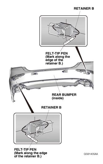
171. Using a felt-tip pen, mark the rear bumper as shown.
