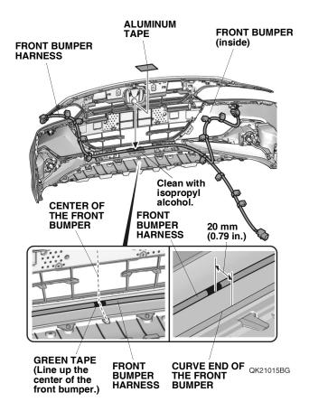
149. Line up the green tape on the front bumper harness with the center of the front bumper, and secure the front bumper harness to the front bumper with one piece of aluminum tape as shown. 150. Using isopropyl alcohol on a shop towel, thoroughly clean the front bumper where the aluminum tape will attach.
