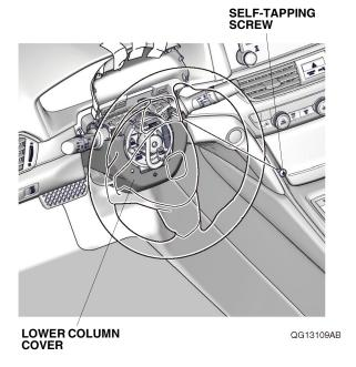
8. Turn the steering wheel 180° counterclockwise, and remove the other self-tapping screw from the lower column cover.
