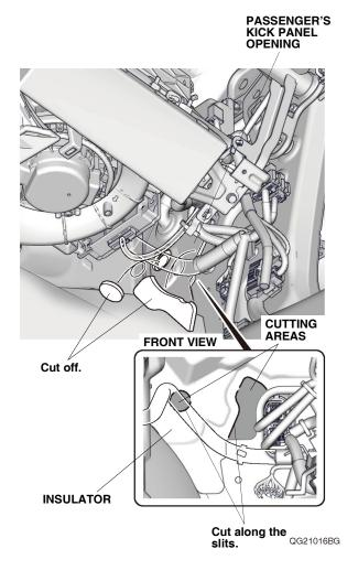
48. Remove the vehicle grommet. Route the subharness through the vehicle panel hole as shown.
