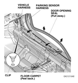
108. Route the parking sensor harness along the vehicle harness.
