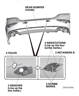
169. Make sure the four sensors are installed properly.
