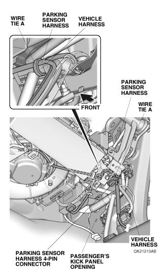
105. Plug the subharness 4-pin connector into the parking sensor harness 4-pin connector.
