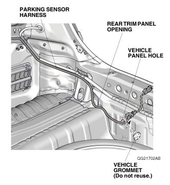
123. Secure the grommet on the parking sensor harness to the vehicle panel hole.
