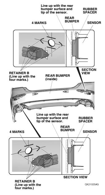
174. Attach the two retainers B to the rear bumper as shown.
