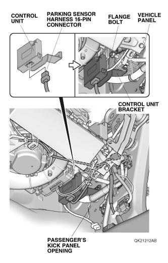
103. Install the control unit to the vehicle panel with one flange bolt.
