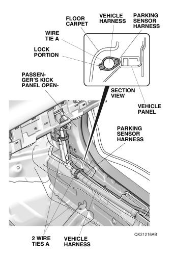
110. Secure the parking sensor harness to the vehicle harness with two wire ties A as shown.
