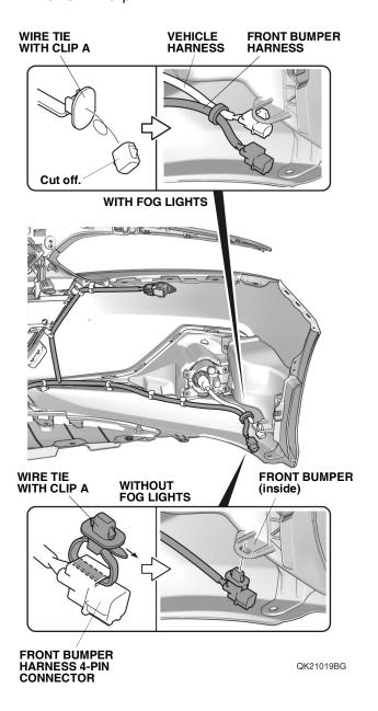
155. With the help of an assistant, bring the front bumper close to the vehicle, and plug the subharness 4-pin connector into the front bumper harness 4-pin connector. Install the front bumper.
