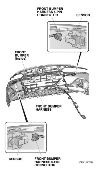
153. Secure the front bumper harness to the ribs on the front bumper with 11 clips on the front bumper harness. Install the front bumper lower cover.
