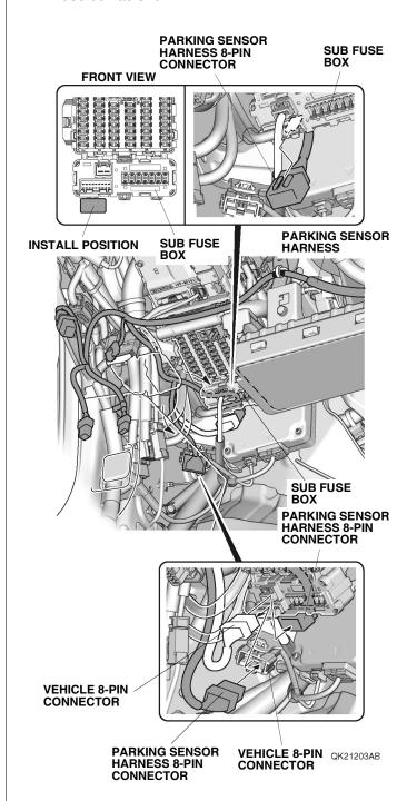
83. Unplug the vehicle 8-pin connector, and plug the parking sensor harness 8-pin connector into the vehicle 8-pin connector. Plug the vehicle 8-pin connector into the parking sensor harness 8-pin connector.
