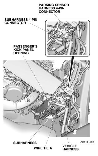
106. Secure the subharness to the vehicle harness with one wire tie A. 107. Pull away the door opening seal, and peel back the floor carpet.
