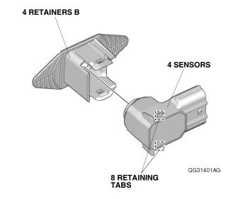
167. Line up the two sensors and two retainers B to the rear bumper as shown.
