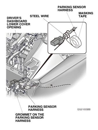
55. Route the parking sensor harness. Remove the masking tape and steel wire.
