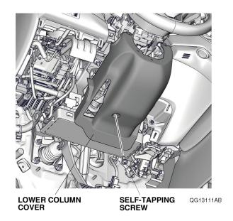
28. Remove the driver's inner dashboard trim and unplug the vehicle connector.
