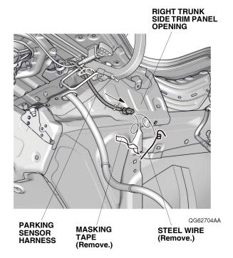
120. Route the parking sensor harness, and secure it to the vehicle panel with two clips on the parking sensor harness.
