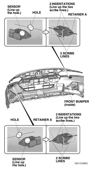
140. Make sure the two sensors are installed properly.
