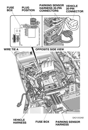
81. Secure the parking sensor harness to the vehicle harness with one wire tie A. Go to step 85.
