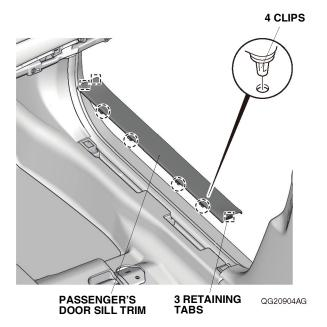
16. Pull away the door opening seal, and remove the passenger's kick panel.
