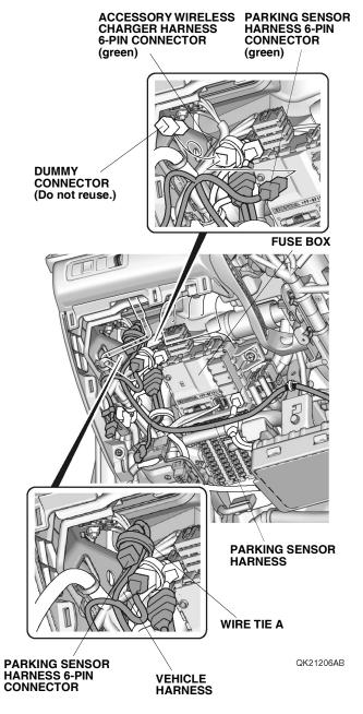
89. Secure the parking sensor harness 6-pin connector to the vehicle harness with one wire tie A. Go to step
