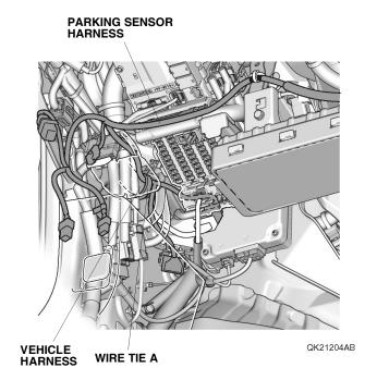
85. If the vehicle is equipped with another accessory harness, follow the plug-in order shown below.
