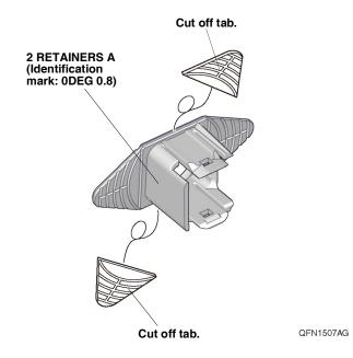
138. Install the two sensors to the two retainers A.
