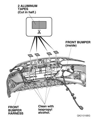
151. Using scissors, cut two pieces of aluminum tape in half, and secure the front bumper harness to the front bumper with the four pieces of aluminum tape as shown.
