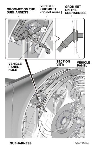
49. Secure the grommet on the subharness to the vehicle panel hole.
