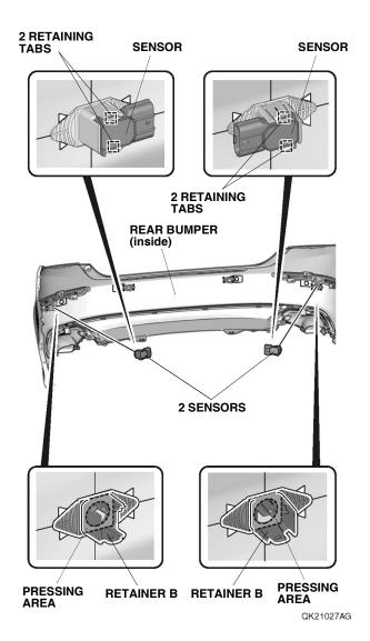
176. Remove the two sensors, and firmly press the two retainers B against the rear bumper.
