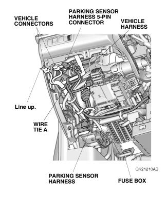
99. Route the parking sensor harness, and secure it to the vehicle harness with two wire ties A.
