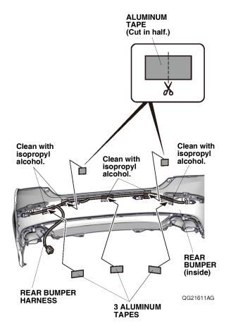
182. Using scissors, cut one piece of aluminum tape in half, and secure the rear bumper harness to the rear bumper with five pieces of aluminum tape as shown.
