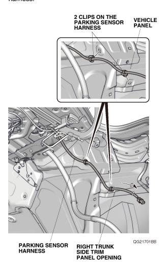
121. Secure the parking sensor harness to the vehicle harness with two wire ties A.
