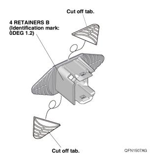
166. Install the four sensors to the four retainers B.
