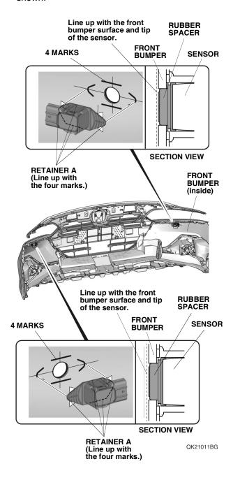
144. Remove the two sensors, and firmly press the two retainers A against the front bumper.
