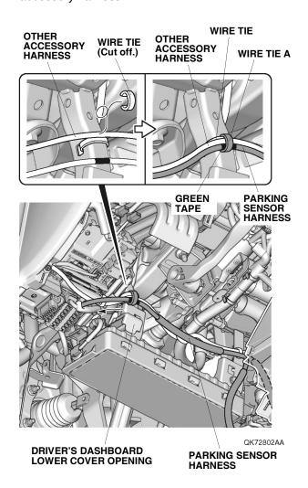
60. Using diagonal cutters, cut off the clip portion of one wire tie with clip B. Line up the branch section of the parking sensor harness with the other accessory clip, and secure the parking sensor harness to the other accessory harness with one wire tie with clip B as shown.
