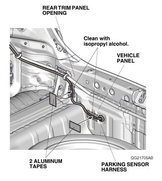
126. Secure the parking sensor harness to the vehicle panel with two pieces of aluminum tape as shown.
