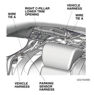
122. Remove the vehicle grommet. Route the parking sensor harness through the vehicle panel hole as shown.
