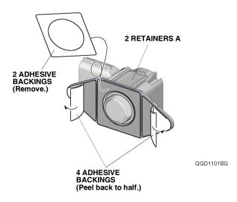
143. Attach the two retainers A to the front bumper as shown.
