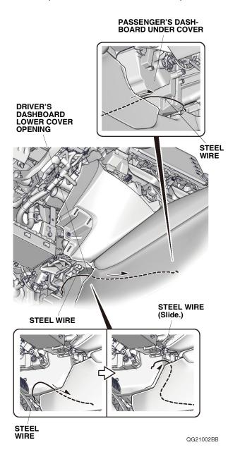
54. Attach the steel wire to the parking sensor harness with masking tape as shown.
