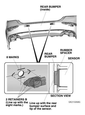
175. Remove the two sensors, and firmly press the two retainers B against the rear bumper.
