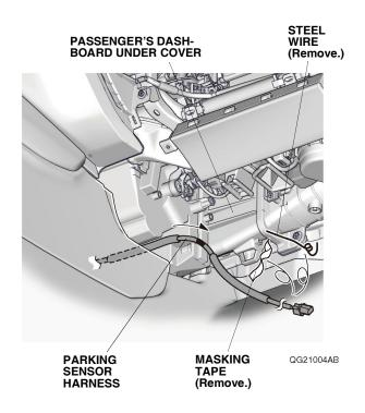
56. Secure the parking sensor harness to the vehicle frame at the green tape on the parking sensor harness with one wire tie A as shown.
