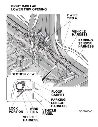
116. Route the parking sensor harness along the vehicle harness, and secure it to the vehicle harness with five wire ties A.
