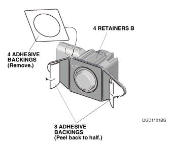
173. Attach the two retainers B to the rear bumper as shown.
