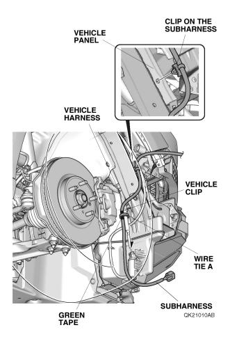
40. Secure the subharness to the vehicle harness with one wire tie A at the green tape on the subharness. Go to step 44.
