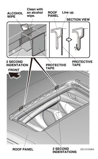
6. Remove the adhesive backings from two pieces of protective tape, and attach one to the roof panel at each second indentation.
