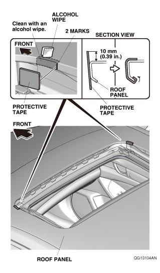
4. Remove the adhesive backings from two pieces of protective tape, and attach one to the roof panel at each of the two marks you made. Wrap 10 mm (0.39 in.) of the protective tape around the lip of the moonroof opening.
