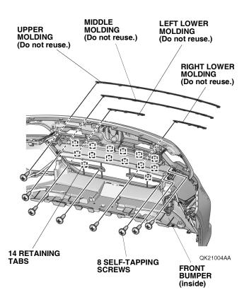
7. Install the upper molding, middle molding, left lower molding, and right lower molding to the front bumper with 14 retaining tabs and the eight self-tapping screws, removed in step 6.
