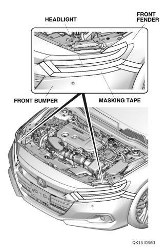
Remove the six self-tapping screws and 17 clips as shown.
