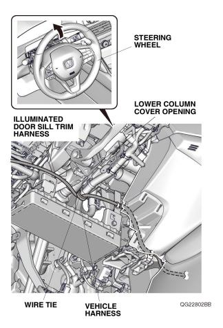
If the vehicle is equipped with the another accessory harness, go to step 36; otherwise, continue with step 35.
