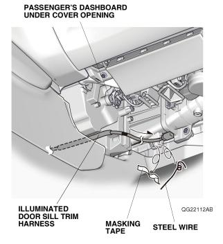
32. Secure the illuminated door sill trim harness to the vehicle frame at the green tape on the illuminated door sill trim harness with one wire tie as shown.
