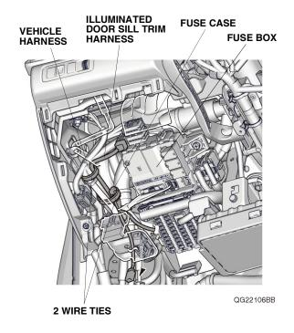
Route the illuminated door sill trim harness as shown, and secure it to the vehicle harness with two wire ties.
