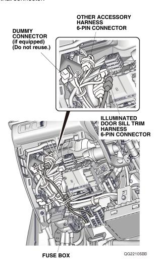
25. Route the illuminated door sill trim harness along the vehicle harness, and secure it and the fuse case to the vehicle harness with two wire ties.
