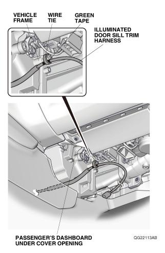
33. Secure the illuminated door sill trim harness to the vehicle frame with one wire tie with clip B as shown. If the vehicle is already equipped with the other accessory harness, cut off the clip from that harness. Secure the illuminated door sill trim harness and other accessory harness to the vehicle frame with one wire tie with clip B.
