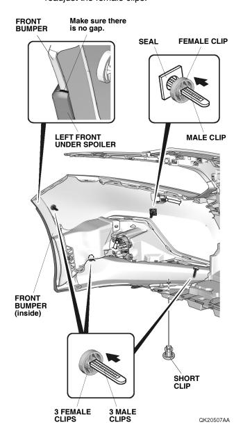
Using diagonal cutters, cut off the excess of the male clips.
