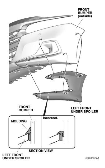
Secure the left front under spoiler to the front bumper with one short clip and four female clips into each male clip as shown.
