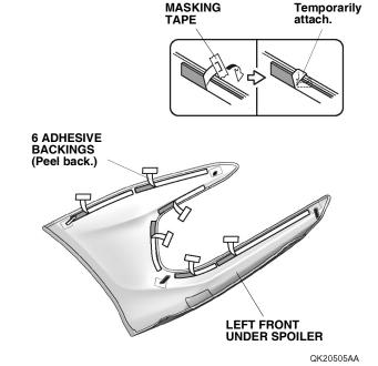
8. Install the left front under spoiler to the front bumper.
