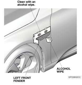
Peel back the adhesive backings, and tape them to the front surface of the left front fender trim with masking tape. Remove the remaining adhesive backings.
