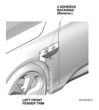
6. Using a rubber roller, apply firm pressure against the left front fender trim and roll from one end to the other. Remove the template.
