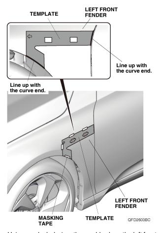
2. Using an alcohol wipe, thoroughly clean the left front fender where the left front fender trim will attach.
