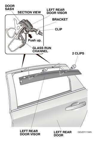
17. Using the two clips, secure the left rear door visor to the brackets as shown. Make sure to push up on the brackets while installing the two clips. NOTE: Be extremely careful when installing the clips; they cannot be reinstalled after installation. 18. Adjust the position of the left rear door visor as shown.
