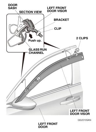
7. Using the two clips, secure the left front door visor to the brackets as shown. Make sure to push up on the brackets while installing the two clips.
