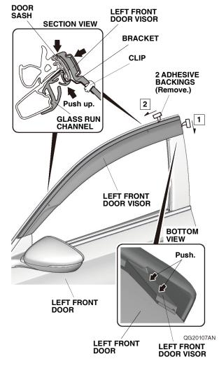
10. Using a soft towel, press and hold the left front door visor against the door sash and left front door for 30 seconds.
