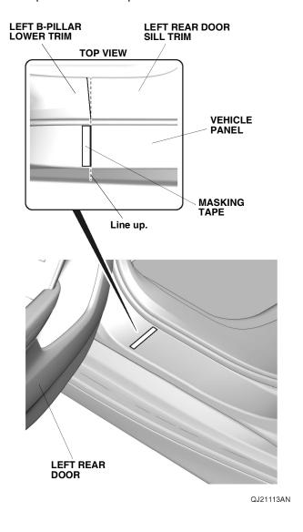
Using an alcohol wipe, thoroughly clean the vehicle panel where the left rear door sill protection film will attach.
