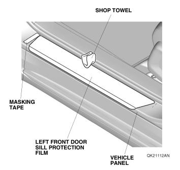
13. Open the left rear door. Attach a piece of masking tape to the vehicle panel as shown.
