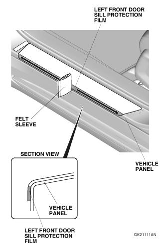
12. Using a shop towel, wipe off the 3M protective tape application solution. Allow the left front door sill protection film to dry thoroughly. Remove the masking tape.
