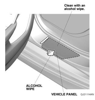
15. Using a spray bottle with the 3M protective tape application solution, spray the vehicle panel where the left rear door sill protection film will attach.
