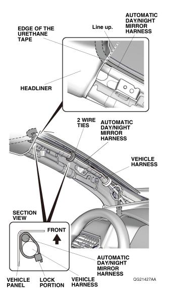
42. Using isopropyl alcohol on a shop towel, thoroughly clean the vehicle panel where the urethane tape will attach.
