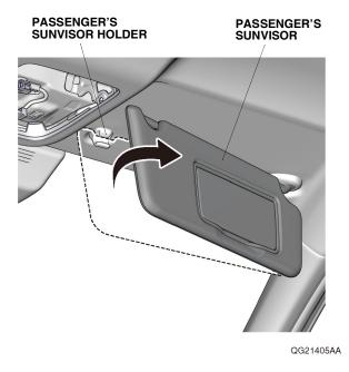
5. Remove the passenger's sunvisor holder by rotating it 45° counterclockwise.
