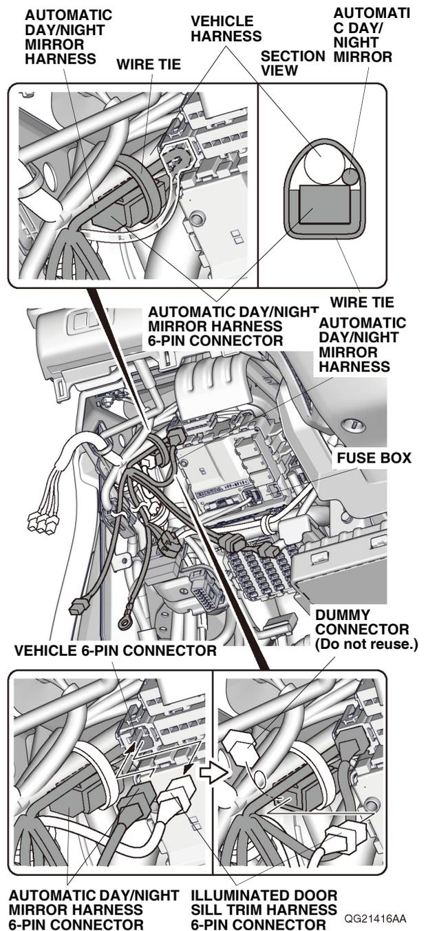
24. Unplug the illuminated door sill trim harness 6-pin connector, and plug the automatic day/night mirror harness 6-pin connector into the vehicle 6-pin connector.
