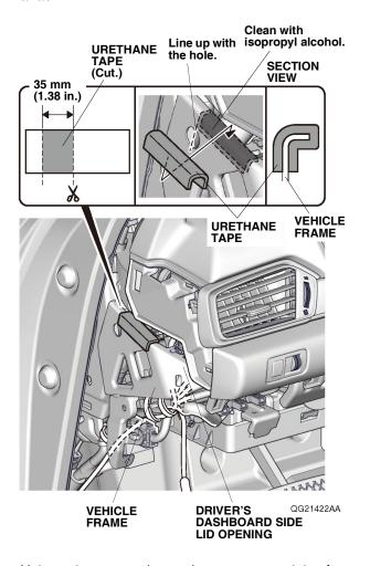
36. Using scissors, cut the urethane tape remaining from step 30 and attach the 35 mm cut piece of urethane tape to the vehicle frame as shown.
