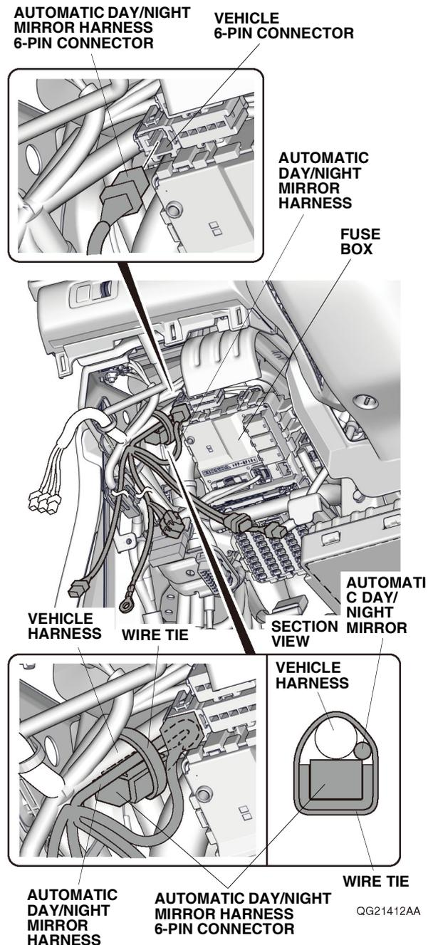
16. Secure the automatic day/night mirror harness 6-pin connector to the vehicle harness with one wire tie as shown. Go to step 26.
