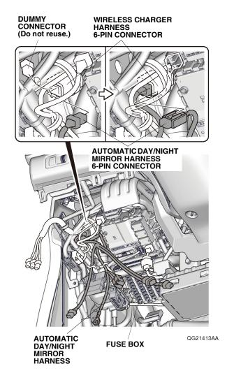
18. Secure the automatic day/night mirror harness 6-pin connector to the wireless charger harness 6-pin connector. Go to step 26.
