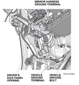
32. Remove the vehicle ground bolt. Secure the automatic day/night mirror harness ground terminal and the vehicle ground terminal with the bolt just removed.
