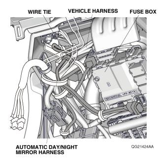
39. Route the automatic day/night mirror harness behind the vehicle harness. Line up the green tape on the automatic day/night mirror harness with the vehicle clip, and secure the automatic day/night mirror harness to the vehicle harness with one wire tie as shown.
