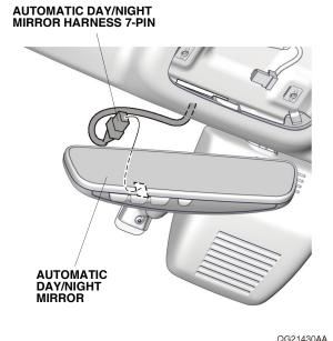
46. Route the automatic day/night mirror harness through the groove in the harness cover, and secure the harness cover to the automatic day/night mirror stay with the two retaining tabs. Slide the harness cover behind the headliner.
