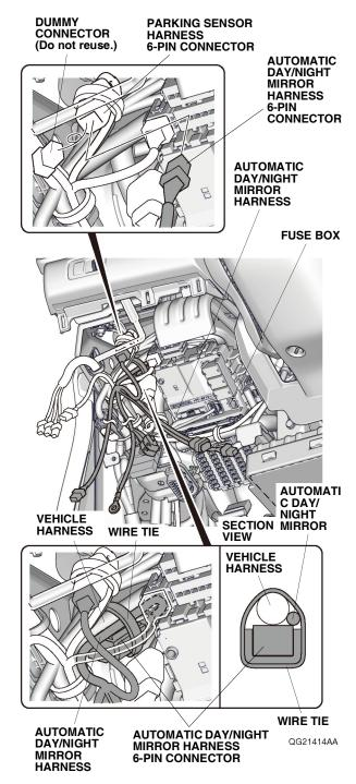
20. Secure the automatic day/night mirror harness 6-pin connector to the vehicle harness with one wire tie as shown. Go to step 26.
