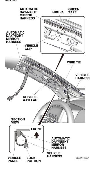
40. Route the automatic day/night mirror harness along the driver's A-pillar. Gently pull back the headliner, and tuck the automatic day/night mirror harness behind the headliner.
