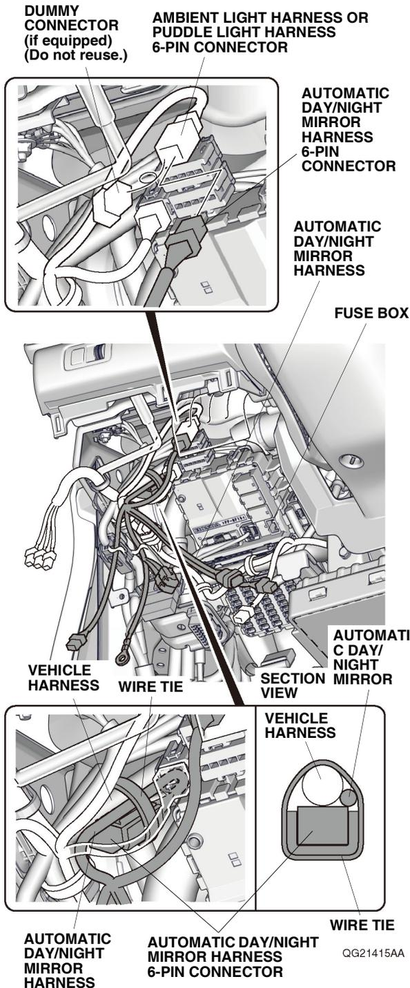
22. Secure the automatic day/night mirror harness 6-pin connector to the vehicle harness with one wire tie as shown. Go to step 26.
