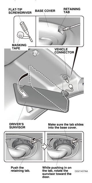
Remove the driver's sunvisor holder by rotating it 45° counterclockwise.
