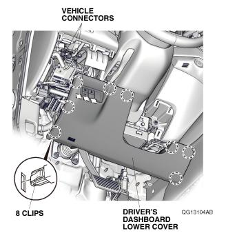
Pull away the door opening seal and remove the driver's dashboard side lid.
