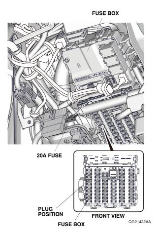
48. Using isopropyl alcohol on a shop towel, thoroughly clean the fuse label where the fuse label will attach. Attach the fuse label (20A OPTION FUSE) to the fuse label on the driver's kick panel as shown.
