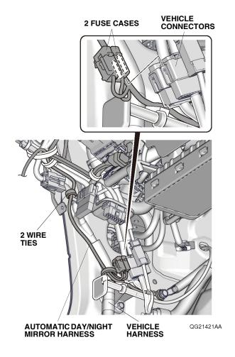
34. Secure the automatic day/night mirror harness to the vehicle harness with two wire ties.
