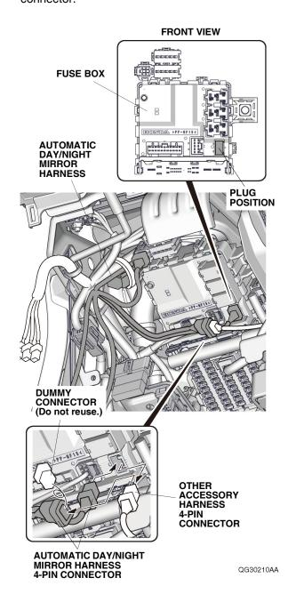
28. Secure the automatic day/night mirror harness to the vehicle harness with three wire ties.
