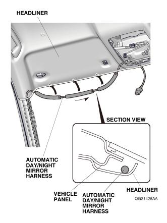
41. Secure the automatic day/night mirror harness to the vehicle harness with two wire ties as shown.
