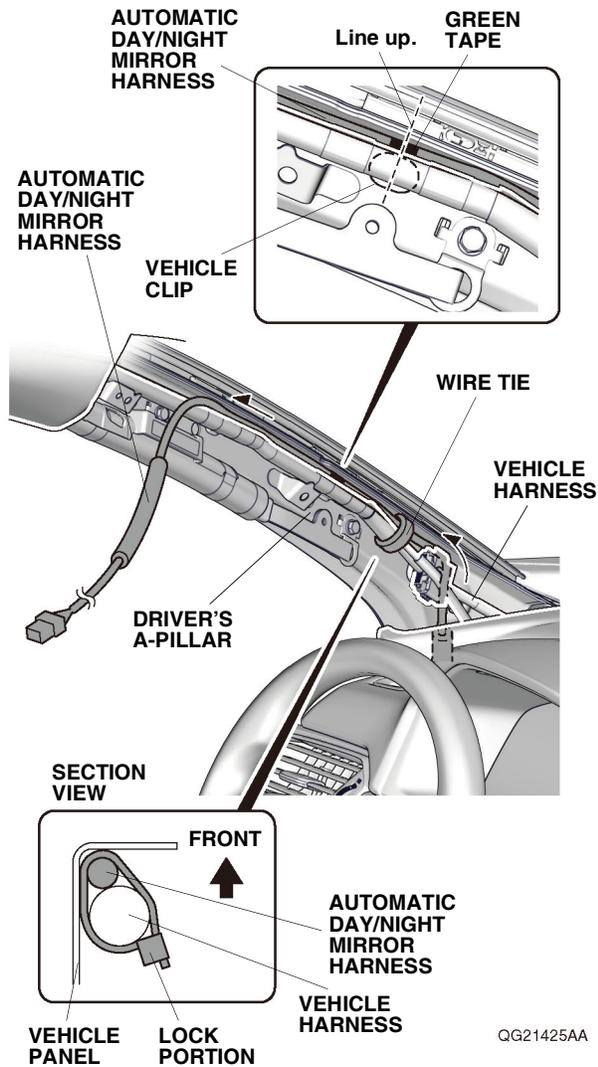
40. Route the automatic day/night mirror harness along the driver's A-pillar. Gently pull back the headliner, and tuck the automatic day/night mirror harness behind the headliner. NOTE: Be careful not to crease the headliner.
