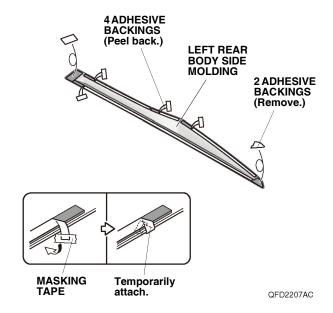
11. Line up the left rear body side molding with the middle template and rear template, and attach it to the left rear door as shown.
