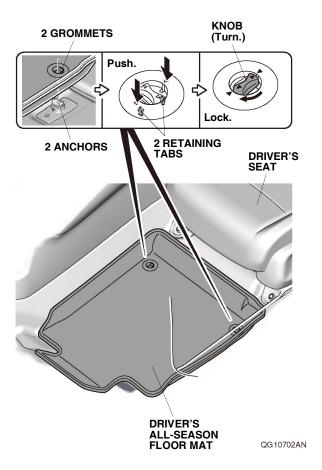
2. Place the grommets in the driver's all-season floor mat over the anchors. Push the grommets into the anchors to secure the retaining tabs, then turn the knobs 90° to secure the driver's all-season floor mat.
