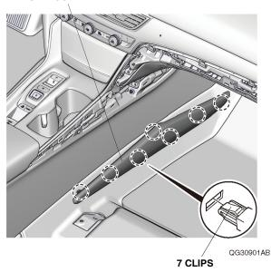
13. Remove the driver's dashboard lower cover and unplug the vehicle connectors.
