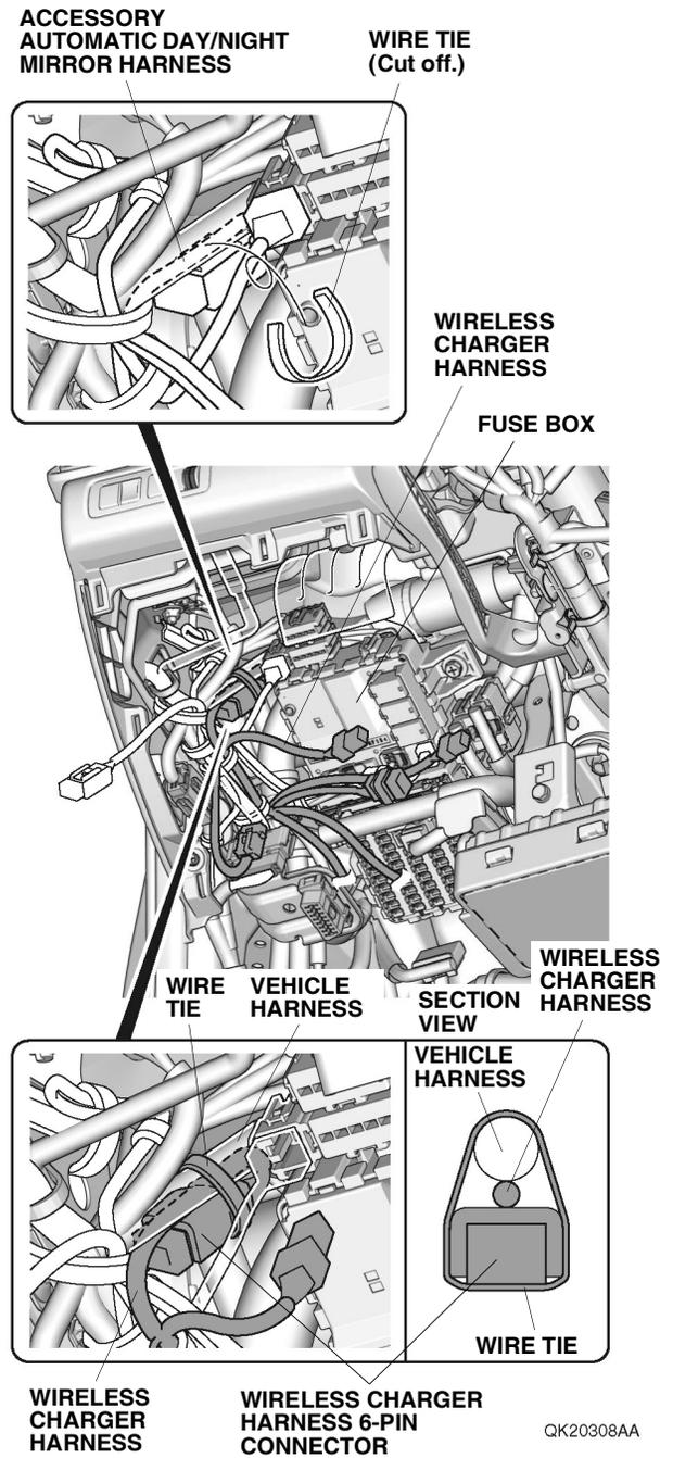
40. Secure the wireless charger harness 6-pin connector to the vehicle harness with one wire tie as shown.
