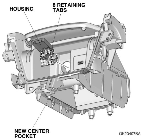
72. Install the accessory power socket in the housing with two retaining tabs.
