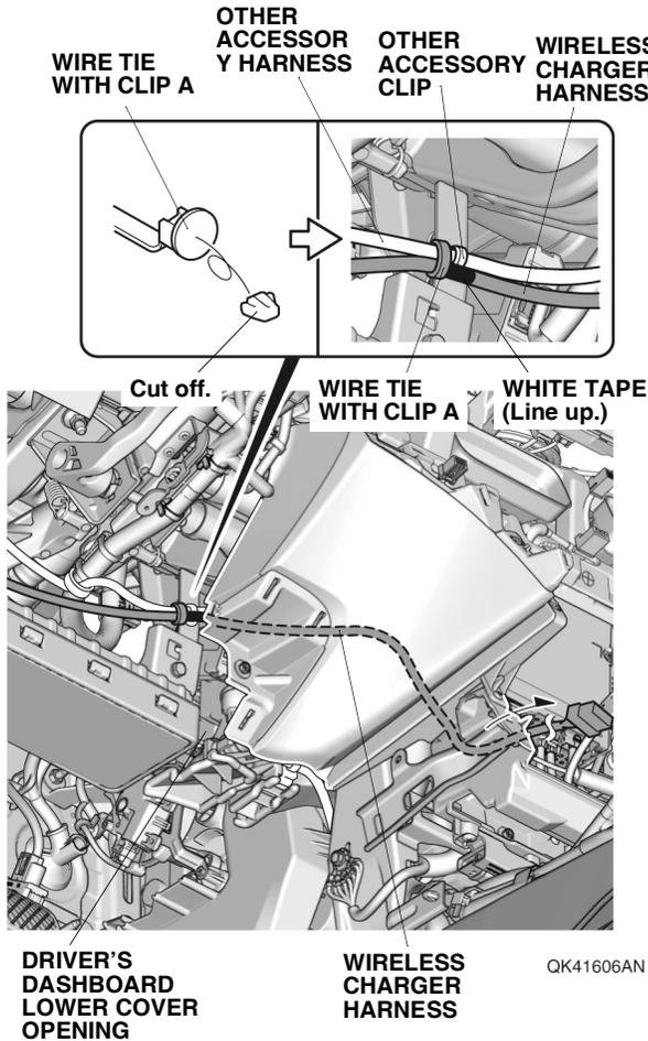
56. Line up the white tape on the wireless charger harness with the other accessory clip, and secure the wireless charger harness to the other accessory harness with one wire tie with clip A as shown.
