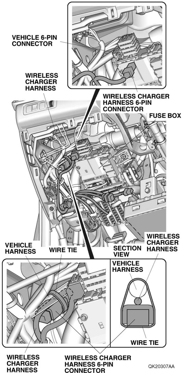
38. Secure the wireless charger harness 6-pin connector to the vehicle harness with one wire tie as shown. Go to step 47.
