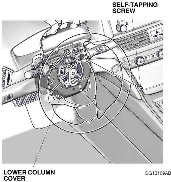
7. Turn the steering wheel 180° counterclockwise, and remove the other self-tapping screw from the lower column cover.
