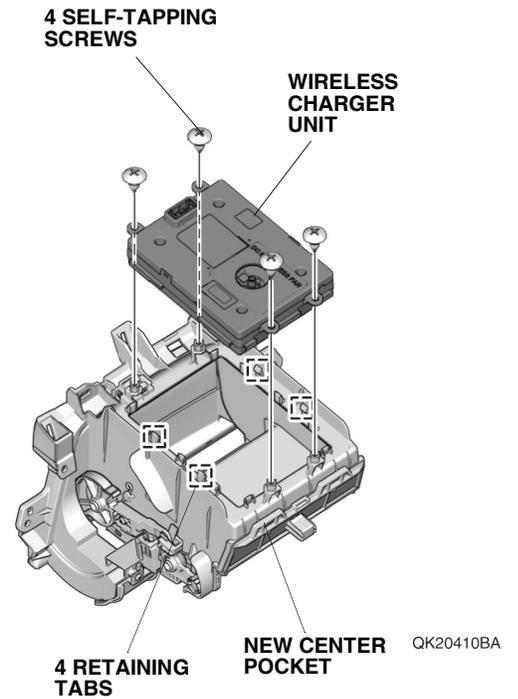
75. Plug the wireless charger harness 7-pin connector into the wireless charger unit.
