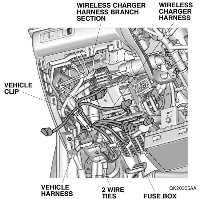
35. Secure the fuse case to the vehicle connectors.
