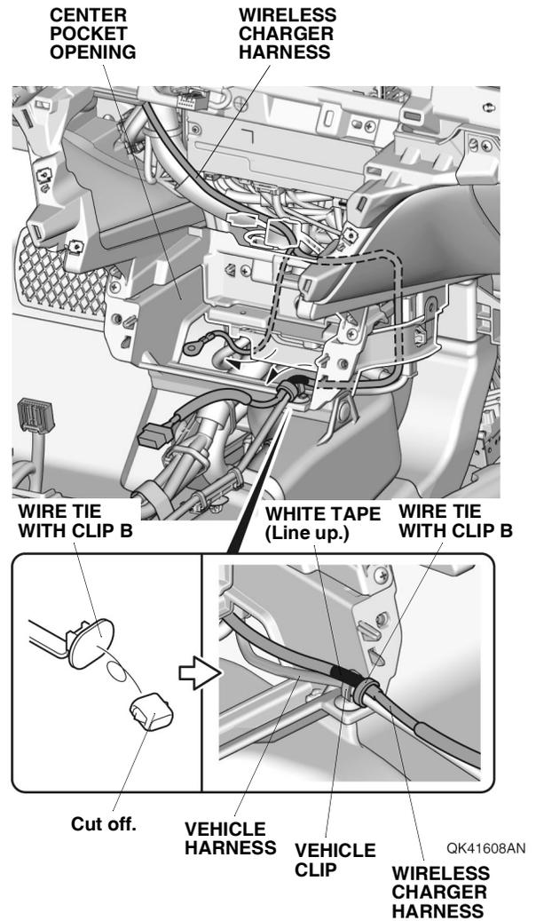
61. Line up the white tape on the wireless charger harness with the vehicle clip, and secure the wireless charger harness to the vehicle harness with one wire tie with clip B as shown.
