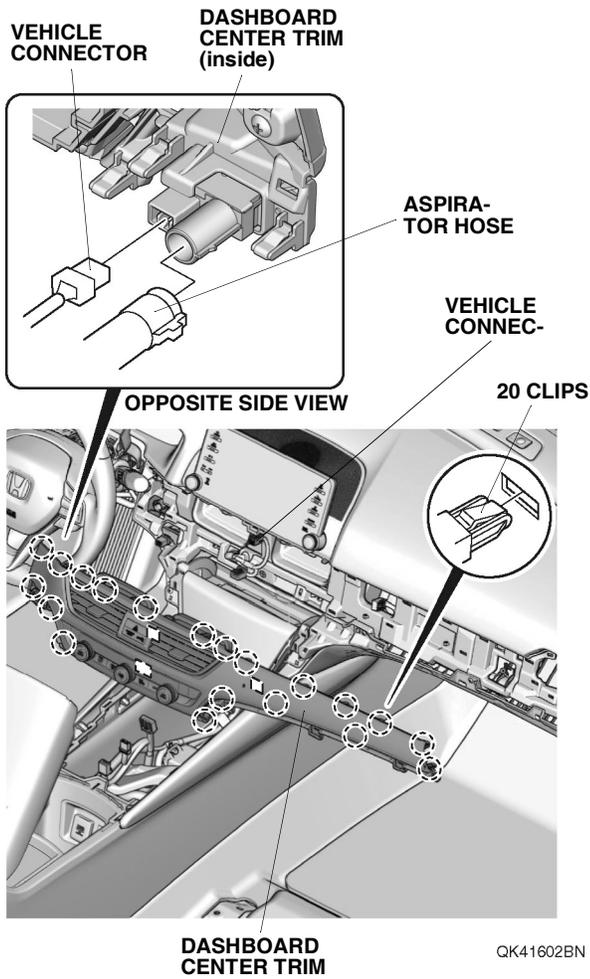
30. Remove the center pocket, and unplug the vehicle connectors.
