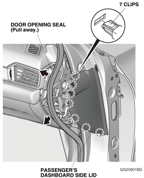
10. Open the glove box and remove the passenger's trim panel. Close the glove box.
