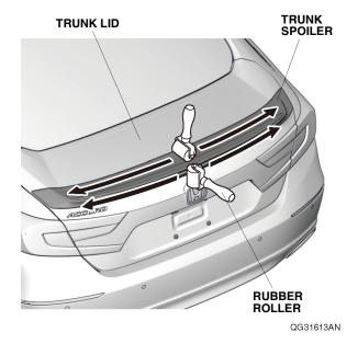
23. Open the trunk lid. Secure the trunk spoiler to the trunk lid with the two flange nuts. Torque the flange nuts to 6.5 lb·ft (8.8 N·m).
