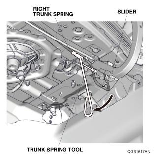
Remove the right trunk spring from the right hinge bracket.
