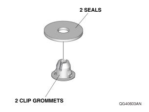
Install the two clip grommets to the two outer holes on the trunk lid.
