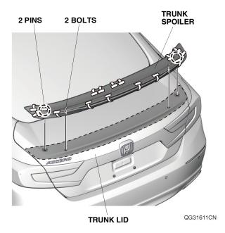
20. Carefully remove the adhesive backings as shown on each side.
