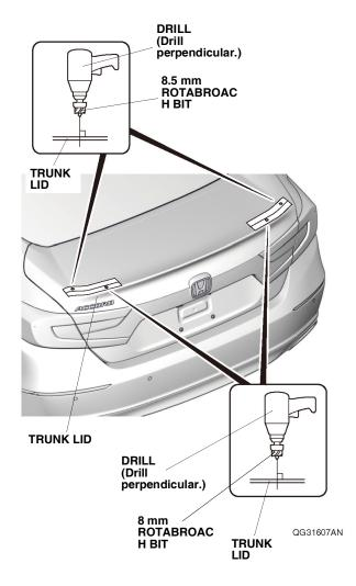
10. While wearing eye protection, use an 8 mm Rotabroach bit to drill the two inner 3 mm holes as shown.
