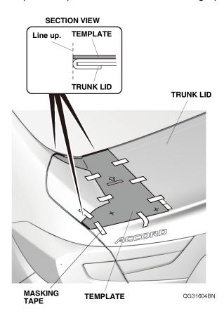
4. Using a felt-tip pen, mark the trunk lid through the template at the two holes on the template.
