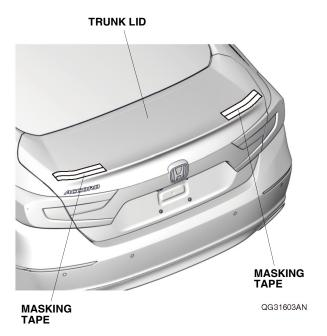
3. Place the template on the left side of the trunk lid, and line up the template with the trunk lid as shown. Tape the template to the trunk lid with masking tape.
