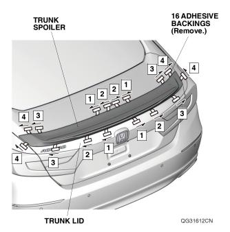
21. Using your hand, firmly press the trunk spoiler against the trunk lid.
