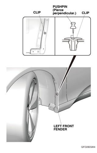
Loosely install the left front splash guard on the left front inner fender and left front fender with one selftapping screw supplied and two self-tapping screws removed in step 2.
