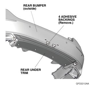
15. Using a rubber roller, apply firm pressure against the rear under trim and roll from one end to the other.
