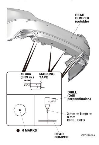
5. While wearing eye protection, enlarge the four drilled holes on the rear bumper to 10 mm with a 10 mm drill hit
