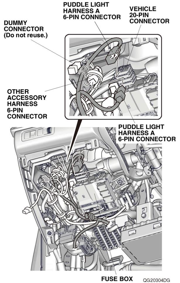
29. Route puddle light harness A along the vehicle harness, and secure it and the fuse case to the vehicle harness with three wire ties.
