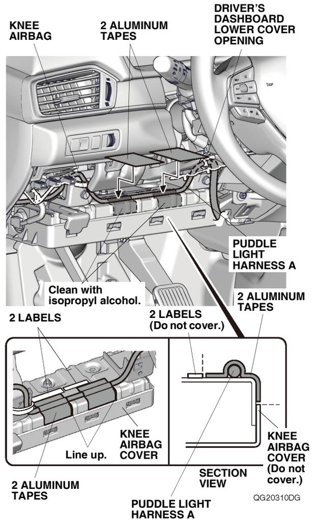
36. Secure puddle light harness A to the knee airbag with two pieces of aluminum tape as shown. Go to step 41.
