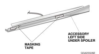
74. Install the accessory left side under spoiler to the vehicle. Remove the masking tape.
