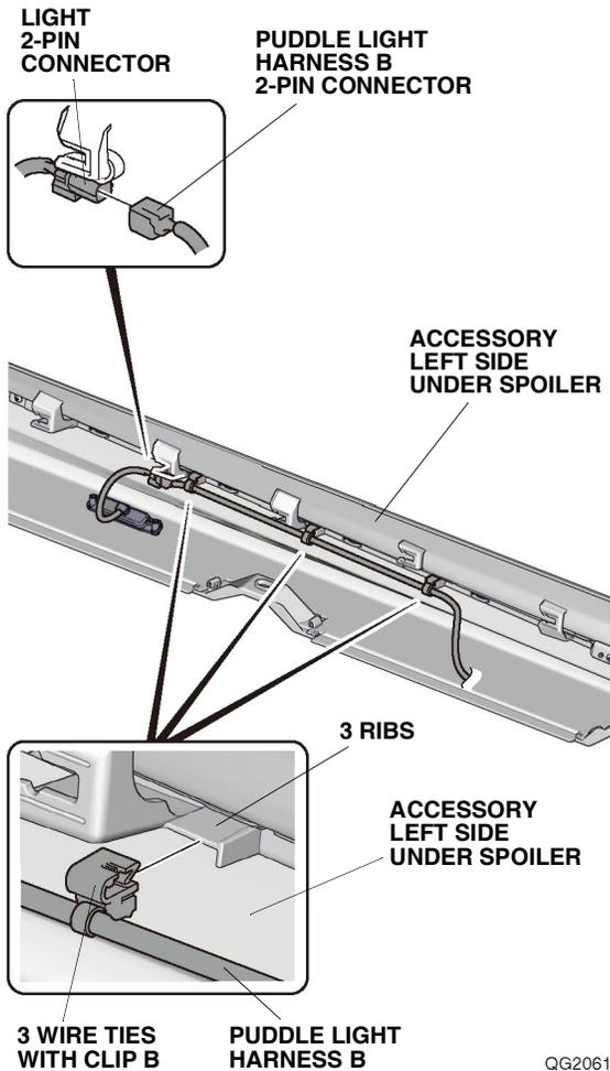
72. Secure the puddle light harness B to the ribs on the accessory left side under spoiler with three wire ties with clip B.
