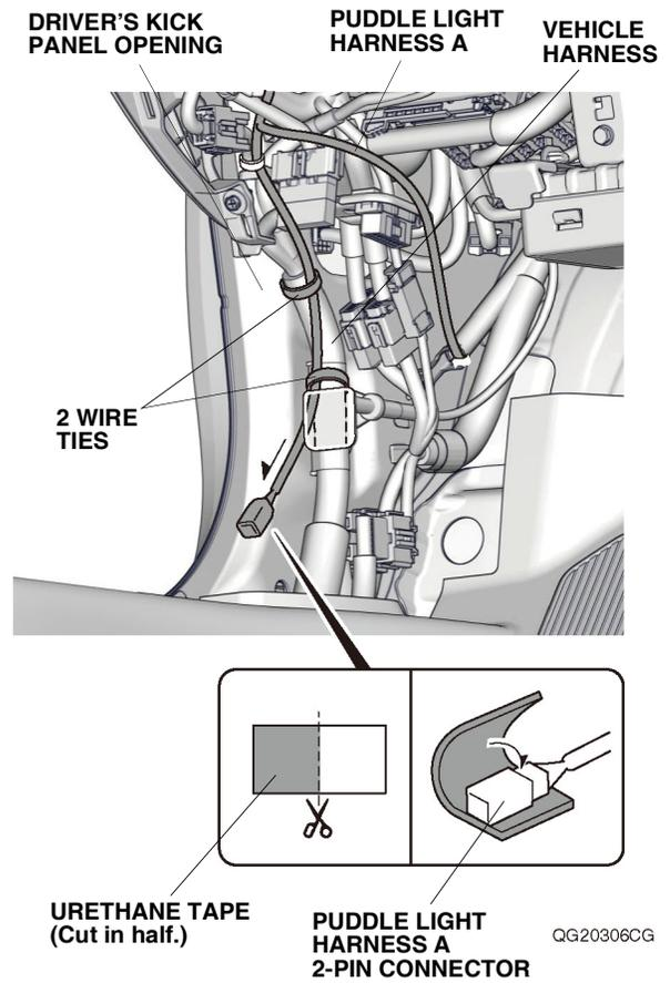
31. Using scissors, cut one urethane tape in half, and attach one piece around the puddle light harness A 2-pin connector.
