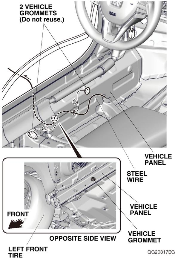
51. Attach the steel wire to the puddle light harness B with masking tape as shown.
