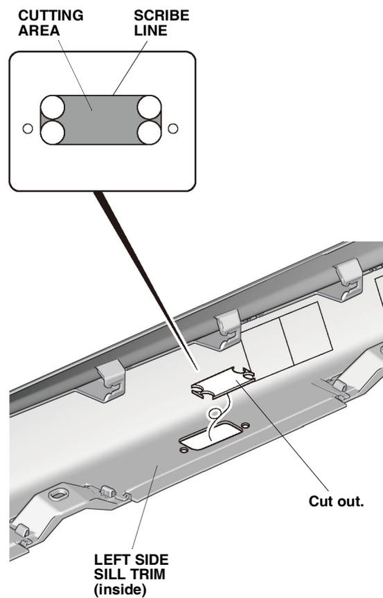
63. Install the light and light trim to the left side sill trim with two self-tapping screws.
