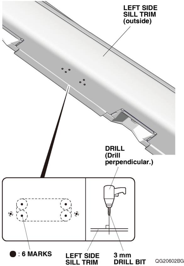
60. While wearing eye protection, enlarge the 3 mm holes on the left side sill trim with a 6 mm drill bit. Remove any burrs. NOTE:
