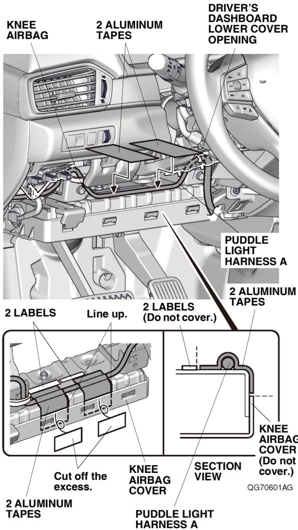
35. Using isopropyl alcohol on a shop towel, thoroughly clean the knee airbag where the aluminum tape will be attached.
