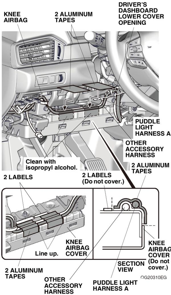
40. Secure puddle light harness A to the knee airbag with two pieces of aluminum tape as shown.
