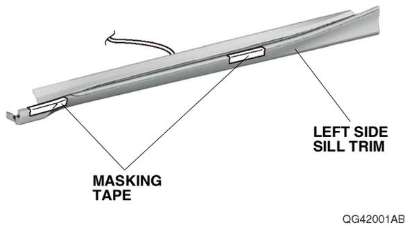
69. Install the left side sill trim to the vehicle. Remove the masking tape.
