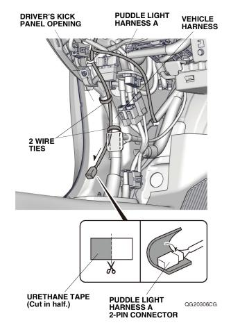
Using scissors, cut one urethane tape in half, and attach one piece around the puddle light harness A 2-pin connector.
