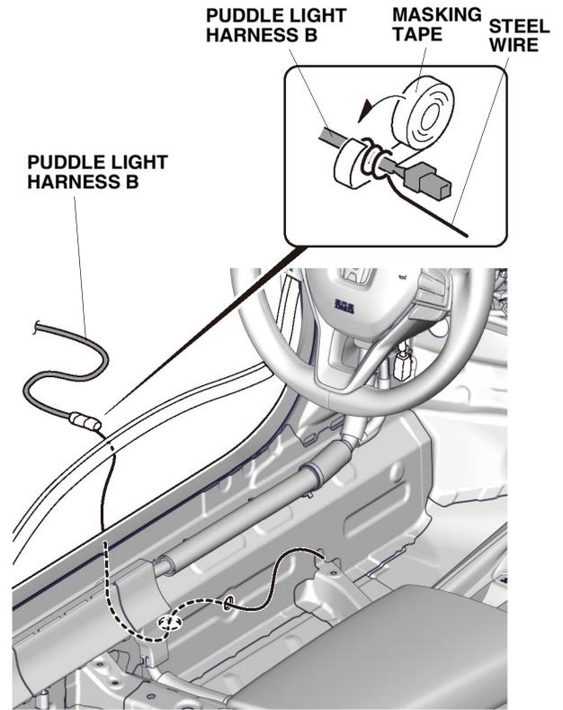
52. Route puddle light harness B. Remove the masking tape and steel wire.
