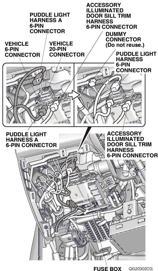
26. Remove the dummy connector from the puddle light harness A 6-pin connector. Plug the accessory illuminated door sill trim harness 6-pin connector into that connector. Go to step 29.
