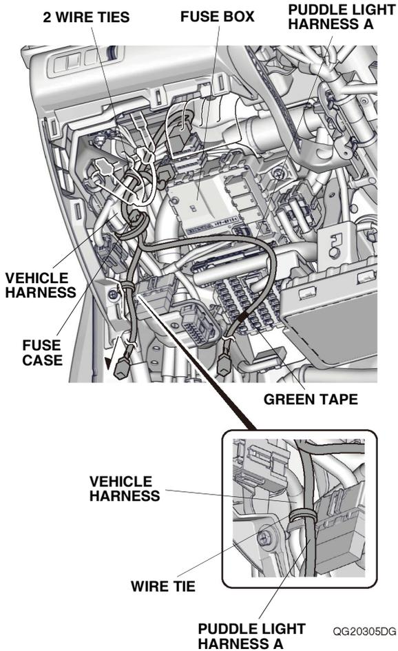
30. Route puddle light harness A along the vehicle harness, and secure it to the vehicle harness with two wire ties.
