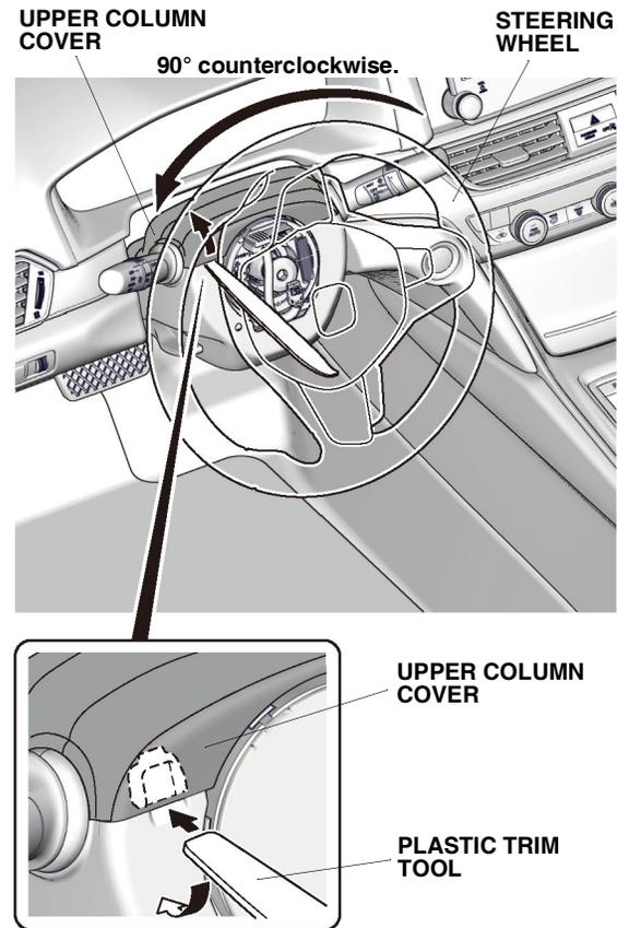
11. Turn the steering wheel 180° clockwise. Using a plastic trim tool, release the upper column cover.
