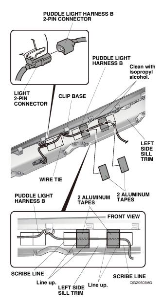
66. Using isopropyl alcohol on a shop towel, thoroughly clean the left side sill trim where the aluminum tape will attach. Secure puddle light harness B to the left side sill trim with two pieces of aluminum tape as shown.
