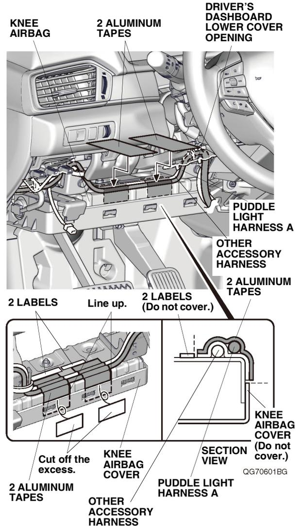
39. Using isopropyl alcohol on a shop towel, thoroughly clean the knee airbag where the aluminum tape will be attached.
