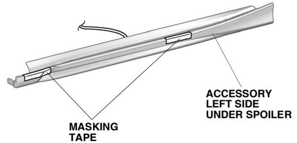
74. Install the accessory left side under spoiler to the vehicle. Remove the masking tape.
