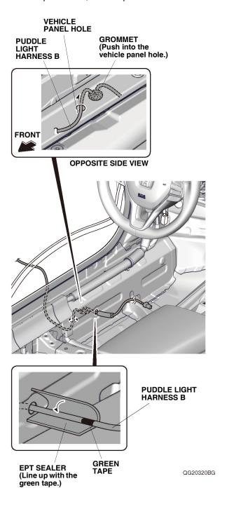
54. Route puddle light harness B wrapped with the EPT sealer as shown, and secure the grommet to the vehicle panel hole.
