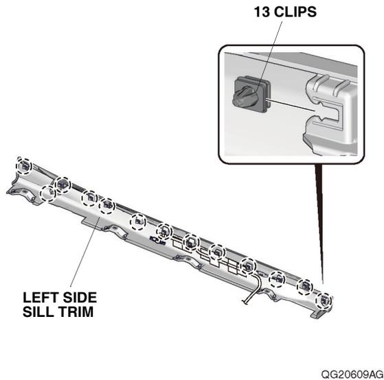
68. To prevent damage from hitting the doors while installing, apply masking tape to the left side sill trim.
