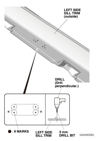
60. While wearing eye protection, enlarge the 3 mm holes on the left side sill trim with a 6 mm drill bit. Remove any burrs.
