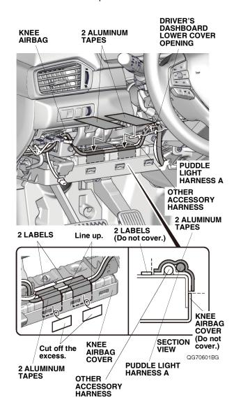
Using isopropyl alcohol on a shop towel, thoroughly clean the knee airbag where the aluminum tape will attached.
