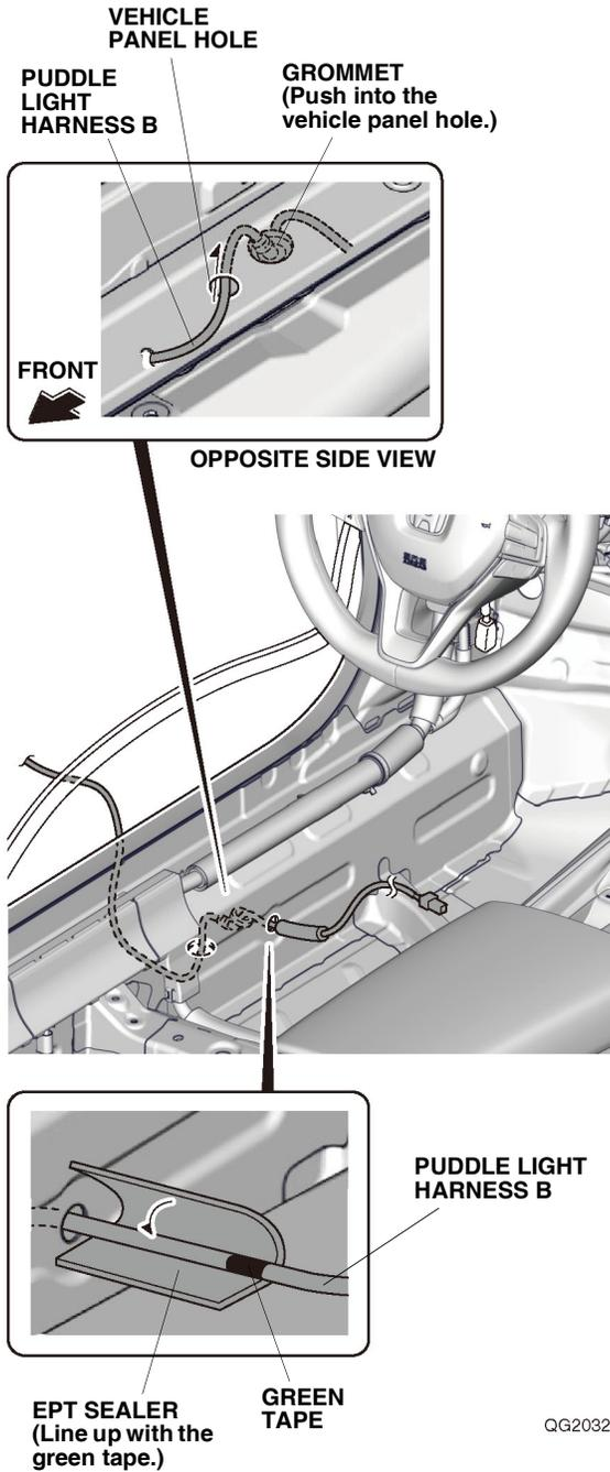
54. Route puddle light harness B wrapped with the EPT sealer as shown, and secure the grommet to the vehicle panel hole.
