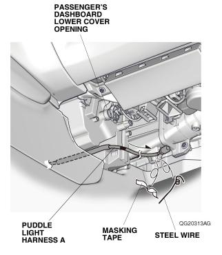
44. Route puddle light harness A as shown, and secure it to the vehicle frame at the green tape on puddle light harness A with one wire tie.
