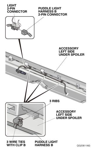
72. Secure the puddle light harness B to the ribs on the accessory left side under spoiler with three wire ties with clip B.
