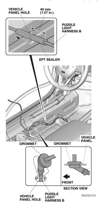
55. Route puddle light harness B along the vehicle harness. Plug the puddle light harness B 2-pin connector into the puddle light harness A 2-pin connector, and secure the 2-pin connectors to the vehicle harness with one wire tie as shown.
