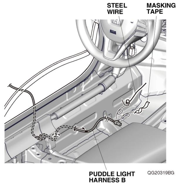
53. Push the grommet on puddle light harness B into the vehicle panel hole, and wrap it with EPT sealer as shown.
