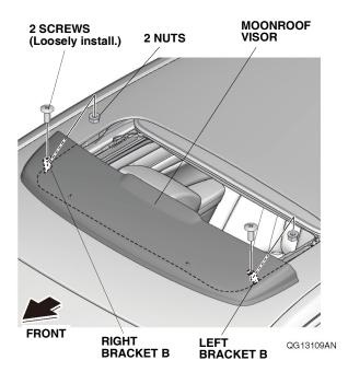
11. Position the moonroof visor with equal spacing on each side. Check that the rubber molding is not twisted or rolled under the moonroof visor.
