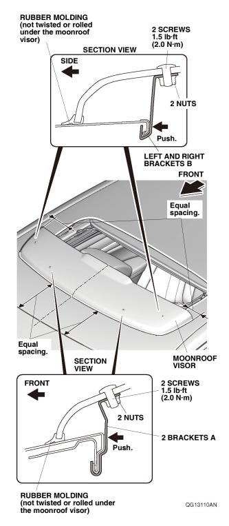
12. Tighten the two screws and two nuts on the front of the vehicle first, then tighten the two screws and two nuts on each side. Tighten while applying pressure so there is no gap between the roof panel and the brackets A and B. Torque the screws to 1.5 lb·ft (2.0 N·m).
