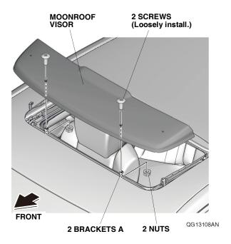
Loosely install the moonroof visor to the left and right brackets B with two screws and two nuts. Remove the strips of masking tape from the left and right brackets B.
