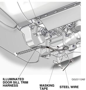
32. Secure the illuminated door sill trim harness to the vehicle frame at the green tape on the illuminated door sill trim harness with one wire tie as shown.
