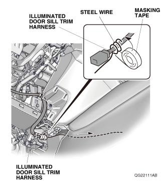
31. Route the illuminated door sill trim harness. Remove the masking tape and steel wire.
