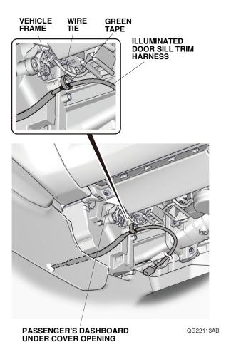
33. Secure the illuminated door sill trim harness to the vehicle frame with one wire tie with clip B as shown. If the vehicle is already equipped with the other accessory harness, cut off the clip from that harness. Secure the illuminated door sill trim harness and other accessory harness to the vehicle frame with one wire tie with clip B.
