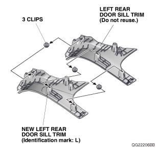
46. Lift the rear seat cushion, and install the new left rear door sill trim on the vehicle panel. Remove the masking tape.
