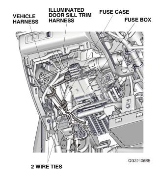
26. Route the illuminated door sill trim harness as shown, and secure it to the vehicle harness with two wire ties.
