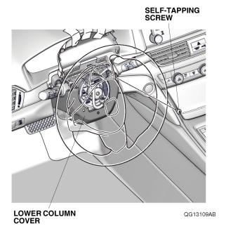
14. Turn the steering wheel 180° counterclockwise, and remove the other self-tapping screw from the lower column cover.
