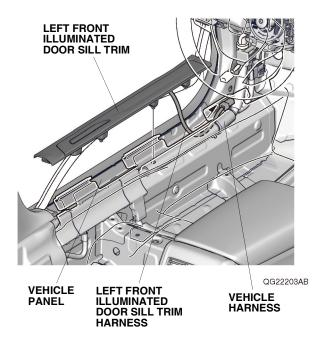
42. Plug the left front illuminated door sill trim 2-pin connector into the illuminated door sill trim harness 2-pin connector, and secure the 2-pin connectors to the vehicle harness with one wire tie as shown.
