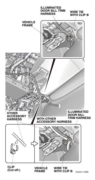
34. Raise the steering wheel. Secure the illuminated door sill trim harness to the vehicle harness with one wire tie.
