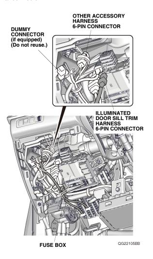
25. Route the illuminated door sill trim harness along the vehicle harness, and secure it and the fuse case to the vehicle harness with two wire ties.
