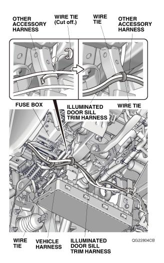
37. Secure the illuminated door sill trim harness to the vehicle frame and vehicle harness with three wire ties.
