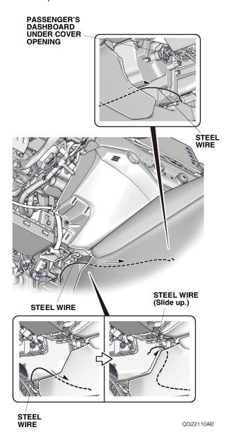
30. Attach the steel wire to the illuminated door sill trim harness with masking tape as shown.
