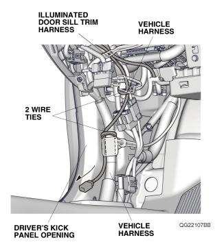
If the vehicle is equipped with another accessory harness, go to step 28; otherwise, continue with step 27.
