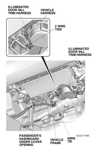
38. Secure the illuminated door sill trim harness to the vehicle harness with three wire ties.
