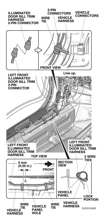
43. Secure the left front illuminated door sill trim harness to the vehicle harness with two wire ties as shown.
