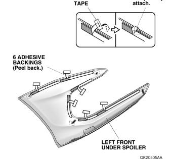
8. Install the left front under spoiler to the front bumper.
