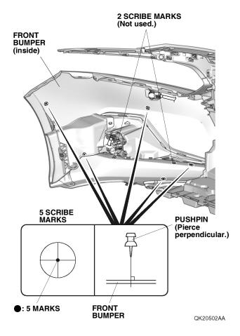
5. While wearing eye protection, drill the five pierced marks on the front bumper to 10 mm. First, drill with a 3 mm drill bit, next, with a 6 mm drill bit, then with an 8 mm drill bit, and finish with a 10 mm drill bit. Remove any burrs.
