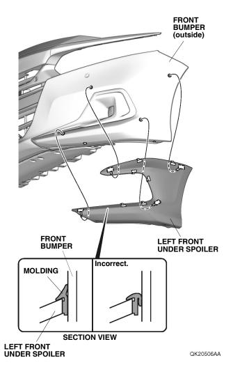
9. Secure the left front under spoiler to the front bumper with one short clip and four female clips into each male clip as shown.
