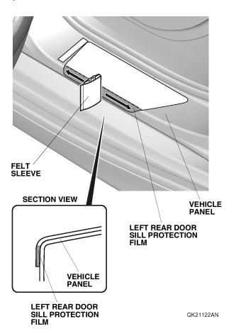
23. Using a shop towel, wipe off the 3M protective tape application solution. Allow the left rear door sill protection film to dry thoroughly. Remove the masking tape.
