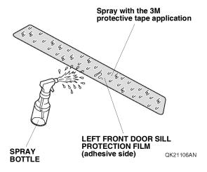
6. Line up the left front door sill protection film with the curve end and masking tape as shown. Attach the left front door sill protection film to the vehicle panel.
