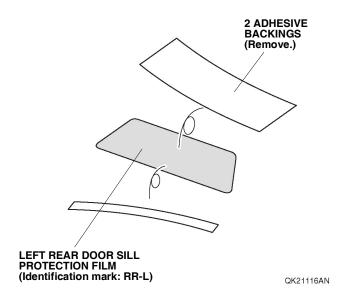
17. Spray the left rear door sill protection film with the 3M protective tape application solution.
