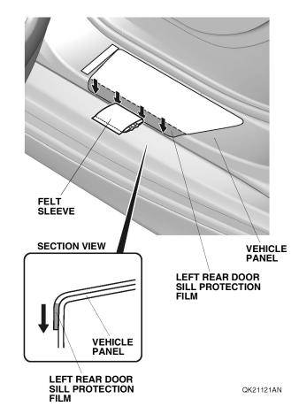
22. Repeat step 20 to set the adhesive of the left rear door sill protection film to the edge of the vehicle panel.
