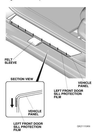
11. Repeat step 9 to set the adhesive of the left front door sill protection film to the edge of the vehicle panel.
