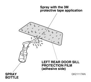
18. Line up the left rear door sill protection film with the curve end and masking tape as shown. Attach the left rear door sill protection film to the vehicle panel.
