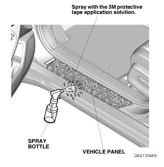
4. Remove the adhesive backings from the left front door sill protection film.
