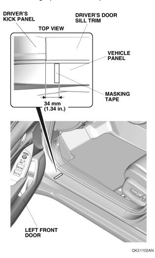
2. Using an alcohol wipe, thoroughly clean the vehicle panel where the left front door sill protection film will attach.
