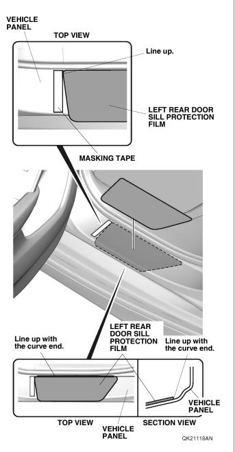
19. Starting from the inside and working outside, use the felt sleeve to smooth out the center of the left rear door sill protection film. Move the felt sleeve in one direction only. If you see an air bubble, stop and gently peel up that section to work out the bubble. Work slowly, and keep pressure against the left rear door sill protection film.
