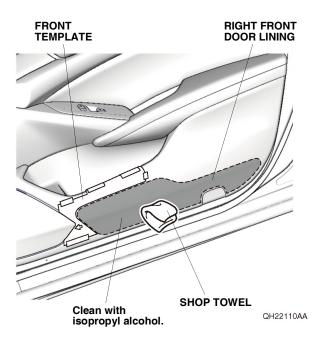
5. Line up the right front door lining cover with the front template. If the vehicle is equipped with courtesy light, make sure there is equal spacing, and attach the right front door lining cover as shown.
