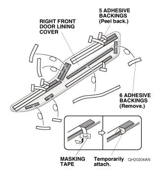
4. Using isopropyl alcohol on a shop towel, thoroughly clean the right front door lining where the right front door lining cover will attach.
