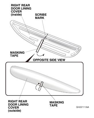
11. Attach masking tape to the right rear door lining cover as shown.
