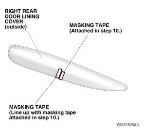
12. Remove masking tape attached in step 10 from the right rear door lining cover.
