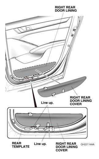
While applying light pressure against the right rear door lining cover, carefully remove the taped adhesive backings.
