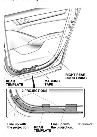
10. Attach masking tape to the right rear door lining cover as shown.
