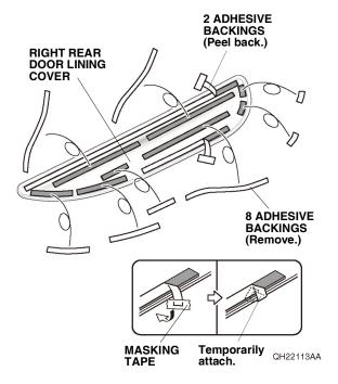
15. Line up the right rear door lining cover with the rear template, and attach it as shown.
