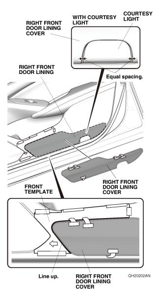
6. While applying light pressure against the right front door lining cover, carefully remove the taped adhesive backings.
