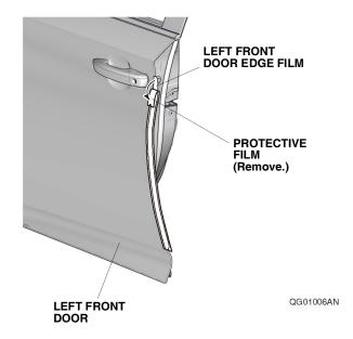
12. Starting from the center and working outward, use your fingers to fold the left front door edge film around the edge of the door. Move your fingers in one direction. Attach the left front door edge film over the seam sealant.
