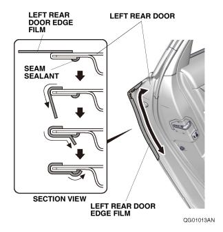
Using a shop towel, wipe the 3M protective tape application solution from the left rear door edge film.
