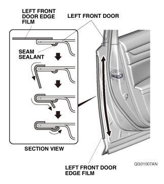
Using a shop towel, wipe the 3M protective tape application solution from the left front door edge film. NOTE: Allow the left front door edge film to dry thoroughly.
