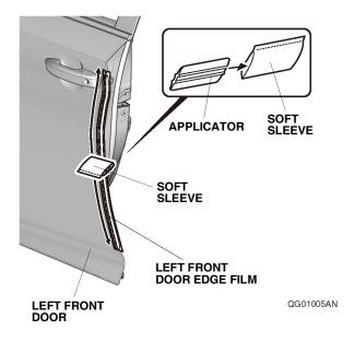
11. Slowly remove the protective film from the left front door edge film.
