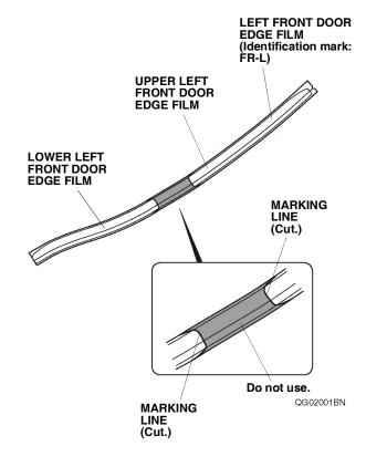
7. Open the left front door again. Peel back about 50 mm (1.97 in.) of adhesive backing from the upper left front door edge film. Line up the upper left front door edge film with the door as shown. NOTE: Check the installation position of the left front
