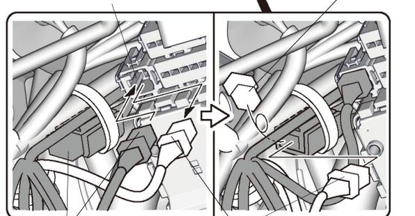
24. Unplug the illuminated door sill trim harness 6-pin connector, and plug the automatic day/night mirror harness 6-pin connector into the vehicle 6-pin connector.
