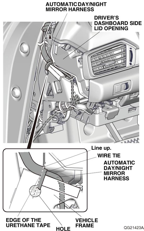
38. Secure the automatic day/night mirror harness to the vehicle harness with one wire tie.
