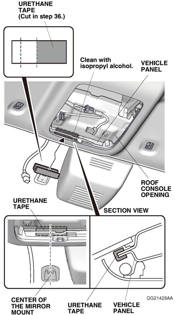
43. Attach the urethane tape cut in step 36 to the vehicle panel as shown.
