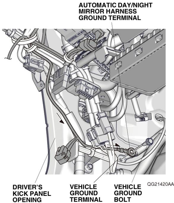
32. Remove the vehicle ground bolt. Secure the automatic day/night mirror harness ground terminal and the vehicle ground terminal with the bolt just removed.
