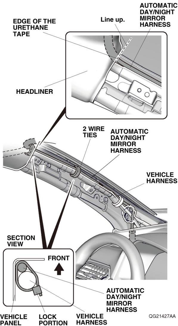
42. Using isopropyl alcohol on a shop towel, thoroughly clean the vehicle panel where the urethane tape will attach.
