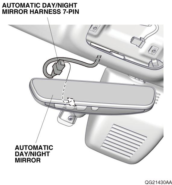
46. Route the automatic day/night mirror harness through the groove in the harness cover, and secure the harness cover to the automatic day/night mirror stay with the two retaining tabs. Slide the harness cover behind the headliner.
