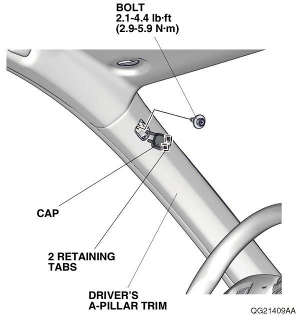
9. Pull away the door opening seal and remove the driver's A-pillar trim.
