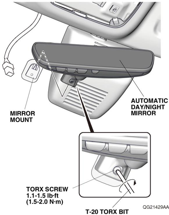
45. Plug the automatic day/night mirror harness 7-pin connector into the automatic day/night mirror.
