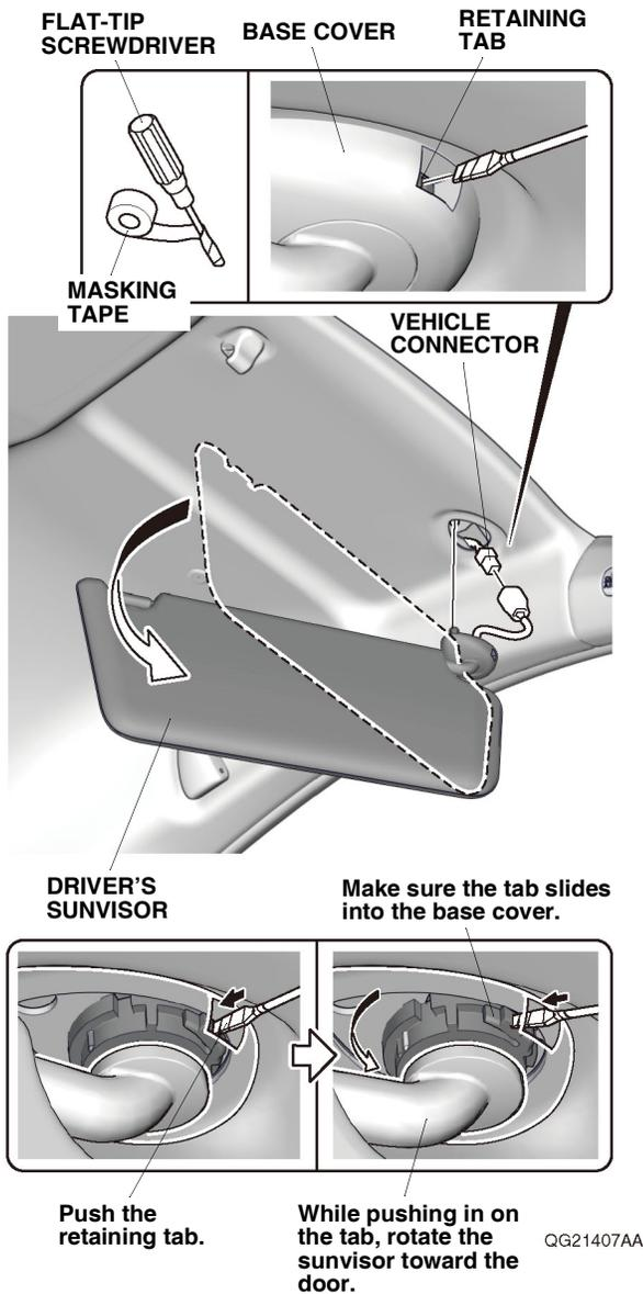
7. Remove the driver's sunvisor holder by rotating it 45° counterclockwise.
