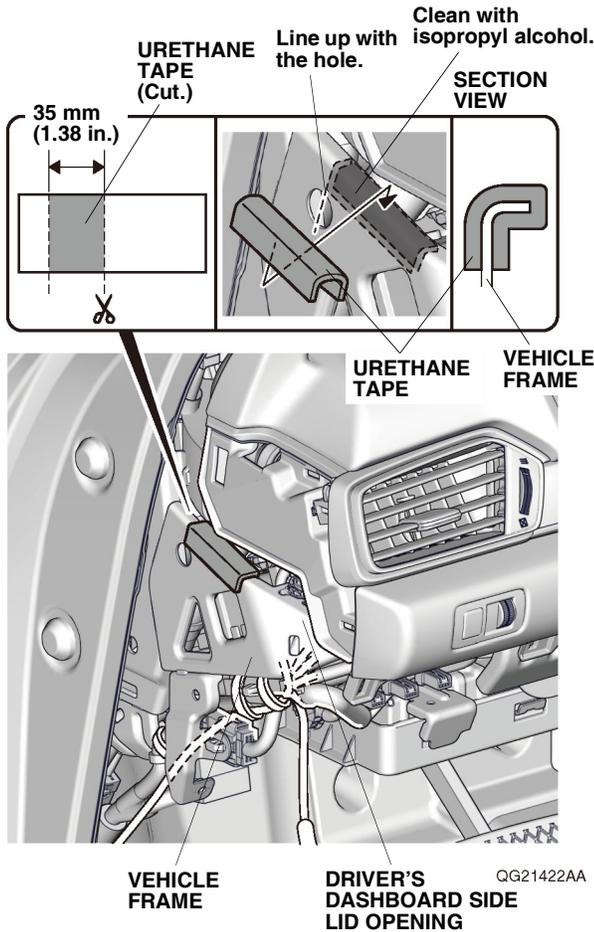
36. Using scissors, cut the urethane tape remaining from step 30 and attach the 35 mm cut piece of urethane tape to the vehicle frame as shown.
