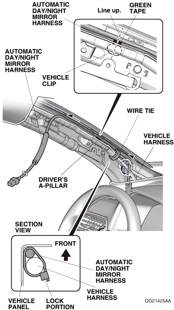
40. Route the automatic day/night mirror harness along the driver's A-pillar. Gently pull back the headliner, and tuck the automatic day/night mirror harness behind the headliner.
