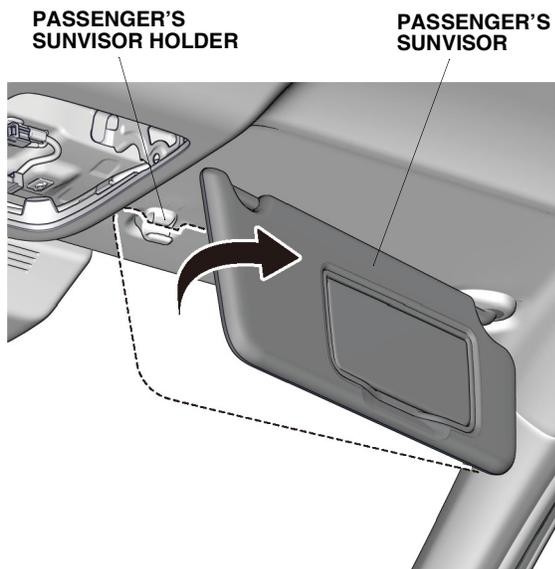
5. Remove the passenger's sunvisor holder by rotating it 45° counterclockwise.
