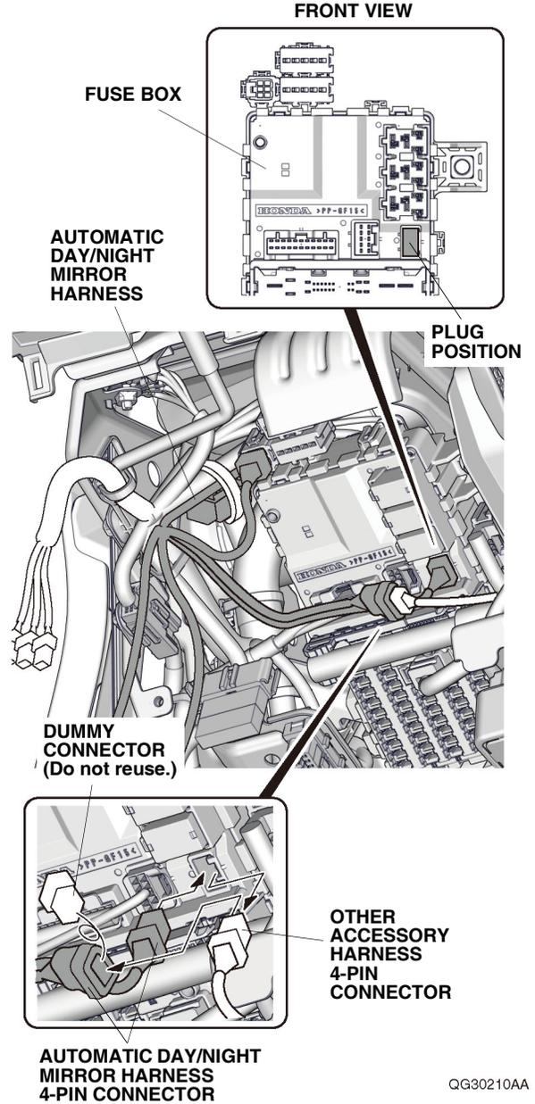
28. Secure the automatic day/night mirror harness to the vehicle harness with three wire ties.
