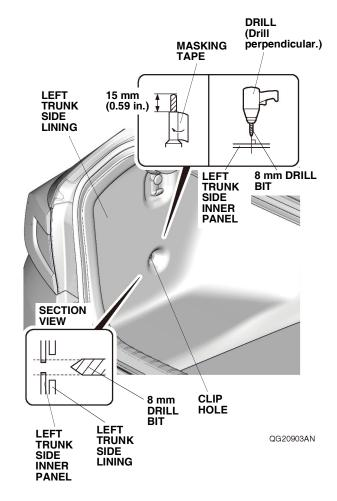
Using a deburring tool, remove all burrs from the hole.
