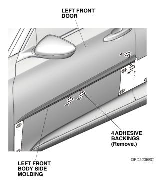
9. Using a rubber roller, apply firm pressure against the left front body side molding and roll from one end to the other.
