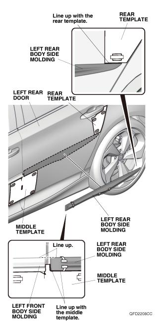
Make sure the edges of the left front body side molding and left rear body side molding are lined up. 13. While applying light pressure against the left rear body side molding, carefully remove the taped adhesive backings.
