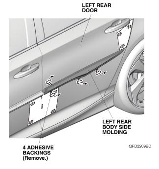
14. Using a rubber roller, apply firm pressure against the left rear body side molding and roll from one end to the other. Remove the templates.
