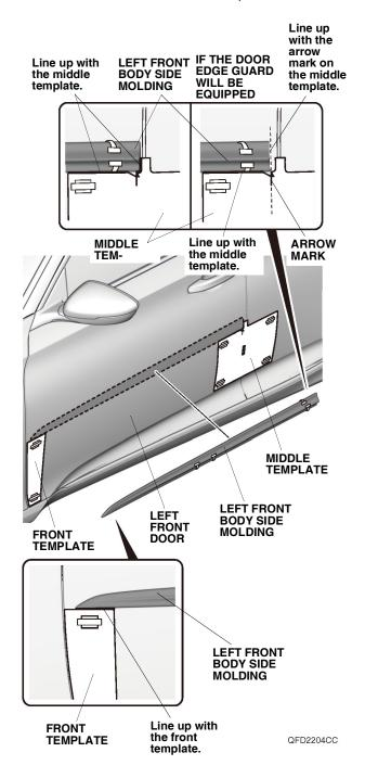
8. While applying light pressure against the left front body side molding, carefully remove the taped adhesive backings.
