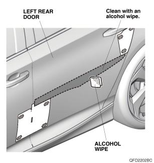
6. Peel back the adhesive backings, and tape them to the front surface of the left front body side molding with masking tape. Remove the remaining adhesive backings.
