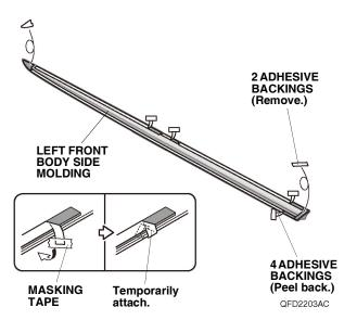
7. Line up the left front body side molding with the front template and middle template, and attach it to the left front door as shown.
