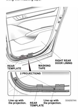
10. Attach masking tape to the right rear door lining cover as shown.
