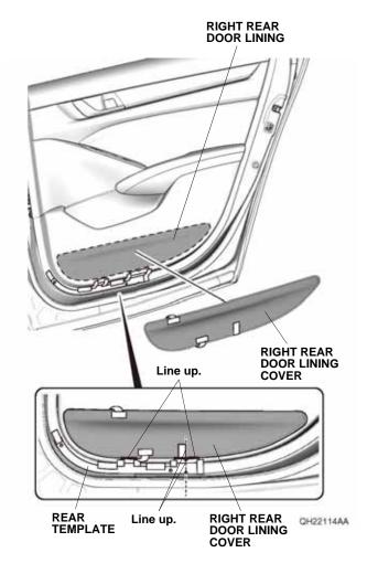
While applying light pressure against the right rear door lining cover, carefully remove the taped adhesive backings.
