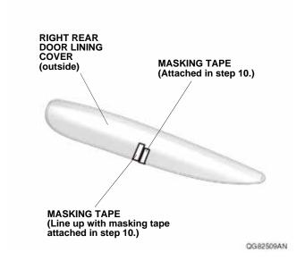
12. Remove masking tape attached in step 10 from the right rear door lining cover.
