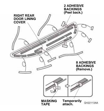
15. Line up the right rear door lining cover with the rear template, and attach it as shown.
