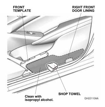
5. Line up the right front door lining cover with the front template. If the vehicle is equipped with courtesy light, make sure there is equal spacing, and attach the right front door lining cover as shown.
