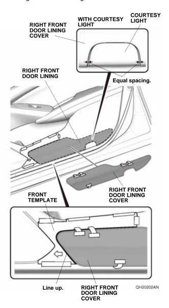
6. While applying light pressure against the right front door lining cover, carefully remove the taped adhesive backings.
