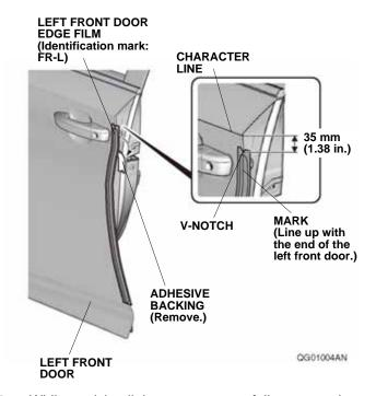
While applying light pressure, carefully remove the adhesive backing. Go to step 10.
