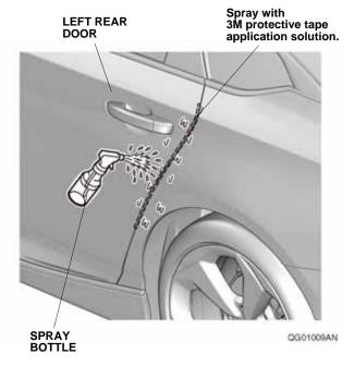
15. Open the left rear door again. Peel back about 50 mm (1.97 in.) of adhesive backing from the left rear door edge film. Line up the left rear door edge film with the left rear door as shown.
