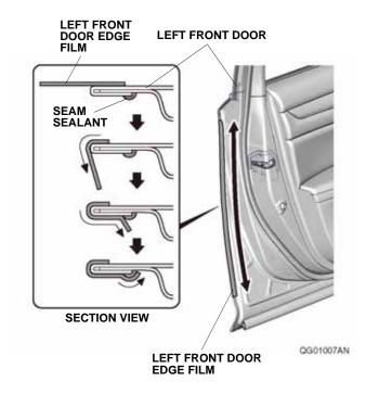
13. Using a shop towel, wipe the 3M protective tape application solution from the left front door edge film. NOTE: Allow the left front door edge film to dry thoroughly.
