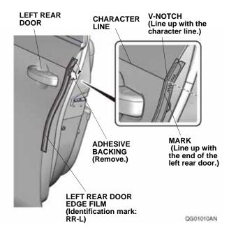
16. While applying light pressure, carefully remove the adhesive backing.
