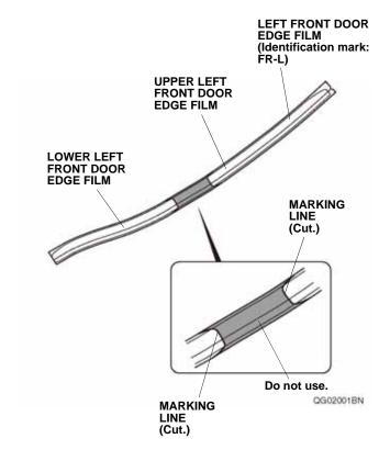
7. Open the left front door again. Peel back about 50 mm (1.97 in.) of adhesive backing from the upper left front door edge film. Line up the upper left front door edge film with the door as shown.
