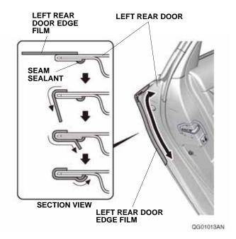
Using a shop towel, wipe the 3M protective tape application solution from the left rear door edge film. NOTE: Allow the left rear door edge film to dry thoroughly.
