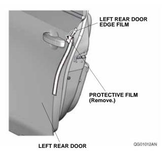
19. Starting from the center and working outward, use your fingers to fold the left rear door edge film around the edge of the door. Move your fingers in one direction. Attach the left rear door edge film over the seam sealant.
