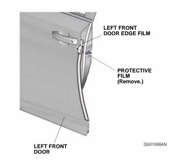
12. Starting from the center and working outward, use your fingers to fold the left front door edge film around the edge of the door. Move your fingers in one direction. Attach the left front door edge film over the seam sealant.
