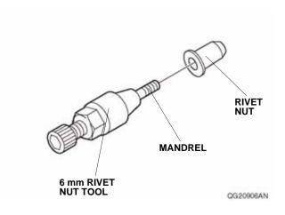
8. Insert the rivet nut into the hole in the vehicle panel, and install the hex wrench on the 6 mm rivet nut tool. NOTE: Make sure to insert the rivet nut in the correct position.
