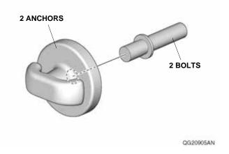
13. Install one anchor into the rivet nut on the vehicle panel as shown. Repeat on the right side of the vehicle.
