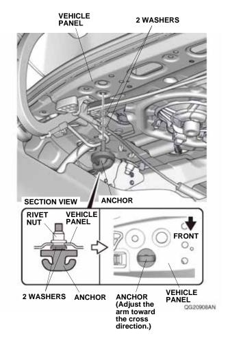
14. Install the cargo net to the anchors and rings as shown.
