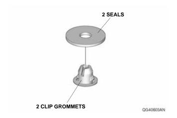
Install the two clip grommets to the two outer holes on the trunk lid.
