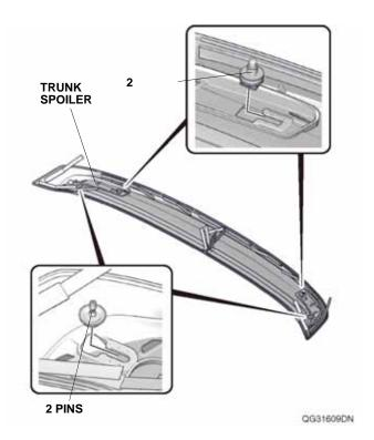
18. Peel back the tabs, and tape them to the front surface of the trunk spoiler with masking tape as shown.
