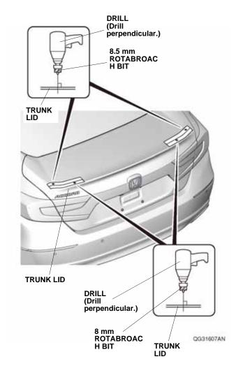
While wearing eye protection, use an 8 mm Rotabroach bit to drill the two inner 3 mm holes as shown.
