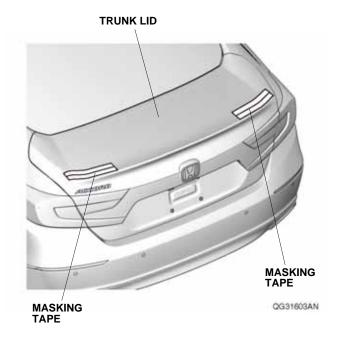
Place the template on the left side of the trunk lid, and line up the template with the trunk lid as shown.
