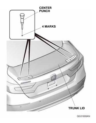
8. While wearing eye protection, drill the four centerpunched marks on the trunk lid with a 3 mm drill bit. NOTE: Make sure to drill the marks perpendicular to the trunk lid.
