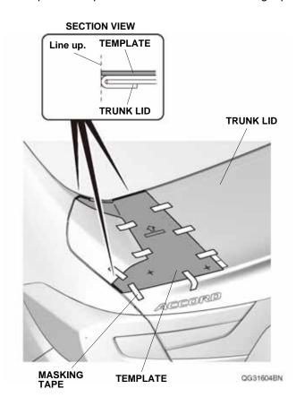
4. Using a felt-tip pen, mark the trunk lid through the template at the two holes on the template.
