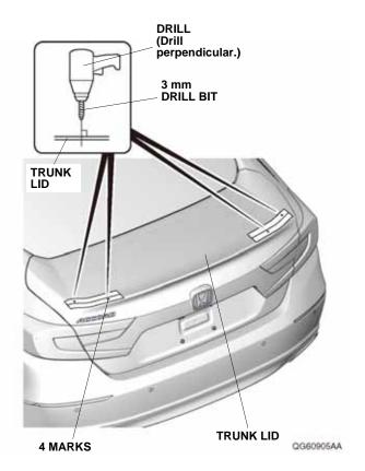
9. While wearing eye protection, use an 8.5 mm Rotabroach bit to drill the two outer 3 mm holes as shown
