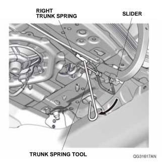
Remove the right trunk spring from the right hinge bracket.
