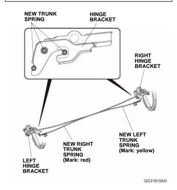
29. Install the new trunk springs to the center clip.
