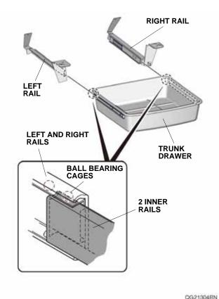
Install the trunk drawer assembly with the six bolts supplied, and torque to 3.0 lb-ft (4.0 N·m).
