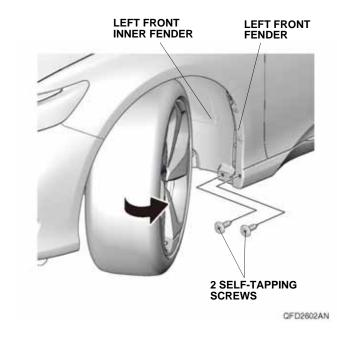
2. Remove the two self-tapping screws from the left front inner fender and left front fender.
