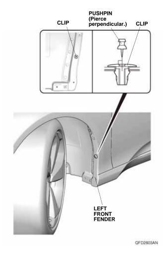
Loosely install the left front splash guard to the left front inner fender and left front fender with one selftapping screw supplied and two self-tapping screws removed in step 2.
