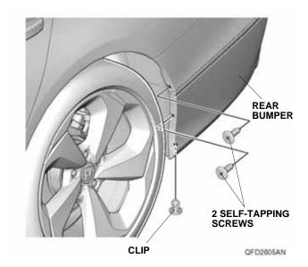
8. Locate the two dimples. Using a pushpin, pierce the rear bumper at the dimples.
