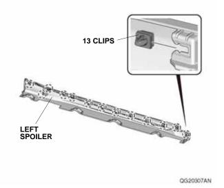
8. To prevent damage from hitting the doors while installing, apply masking tape to the left spoiler.
