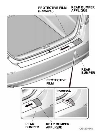
11. Repeat step 8 at the center of the lower section on the rear bumper applique.
