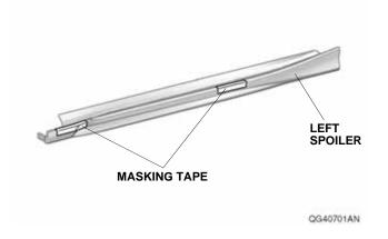
9. Install the left spoiler to the vehicle panel with the 13 clips. Remove the masking tape.
