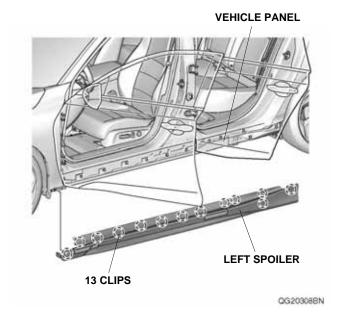
10. Close the left doors. Secure the left spoiler to the vehicle panel with the four clips removed in step 3.
