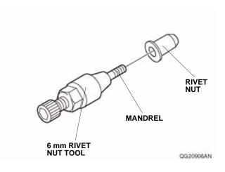
Insert the rivet nut into the hole in the vehicle panel, and install the hex wrench on the 6 mm rivet nut tool. NOTE: Make sure to insert the rivet nut in the correct position.
