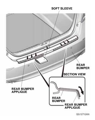
13. Using a shop towel, wipe off the 3M protective tape application solution. Allow the rear bumper applique to dry thoroughly. Remove the masking tape.
