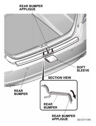
12. Repeat step 9 at the left and right sides of the lower section on the rear bumper applique.
