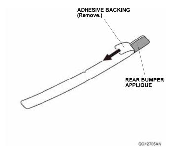
5. Spray the rear bumper applique with the 3M protective tape application solution.
