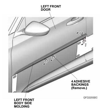
9. Using a rubber roller, apply firm pressure against the left front body side molding and roll from one end to the other.
