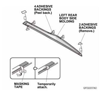
11. Line up the left rear body side molding with the middle template and rear template, and attach it to the left rear door as shown.
