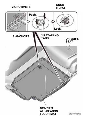
Place the grommets in the driver's all-season floor mat over the anchors. Push the grommets into the anchors to secure the retaining tabs, then turn the knobs 90° to secure the driver's all-season floor mat. 3. Place the passenger's all-season floor mat as shown.
